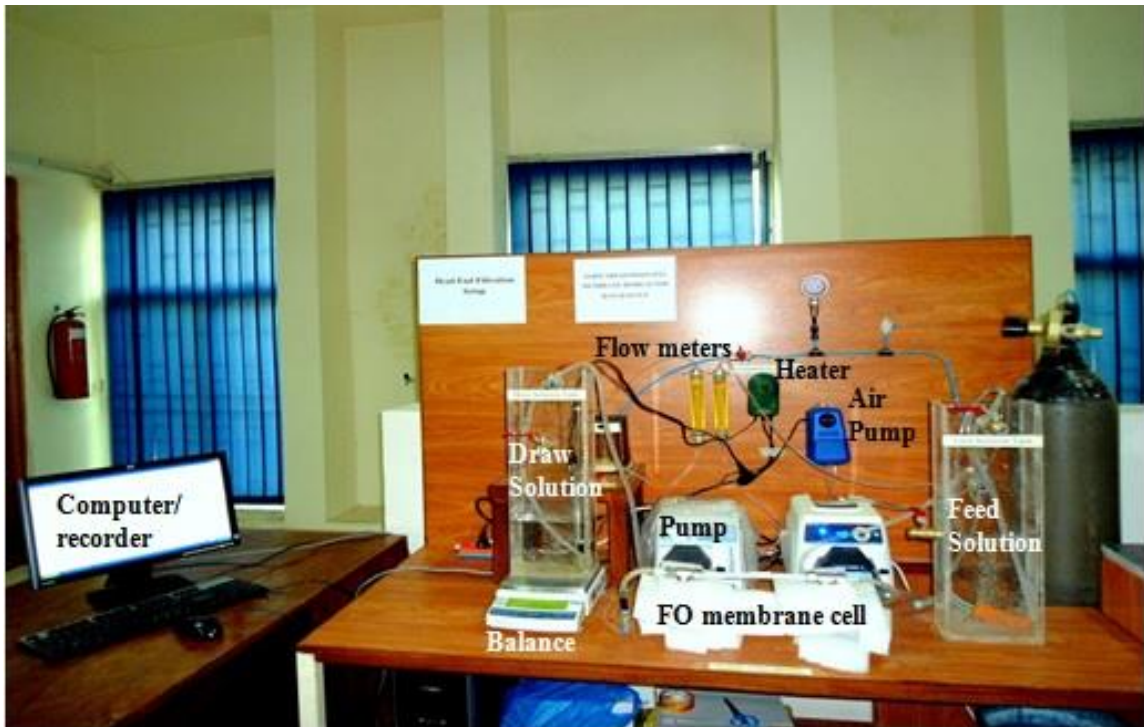
Figure 3.4: Laboratory scale batch FO process setup
