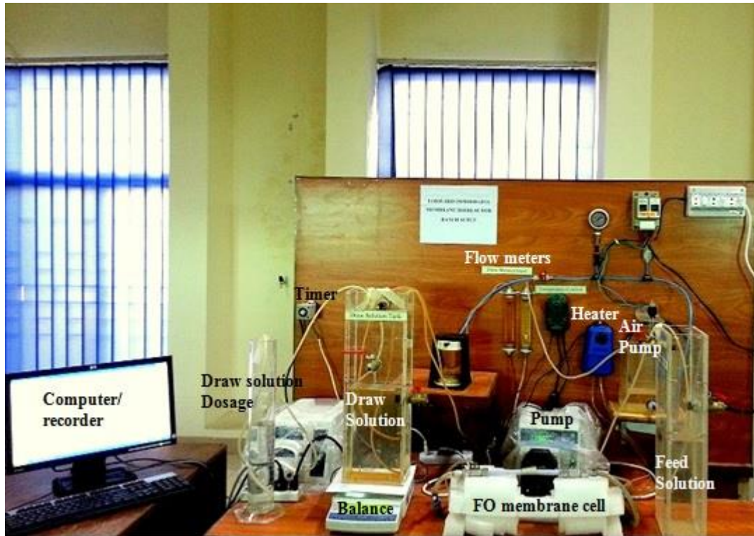
Figure 3.6: Laboratory scale semi-continuous FO process setup
