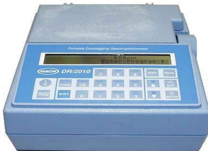
Figure-3.6: Hach digital spectrophotometer (DR 2010) for measuring P- \text{PO}_4
