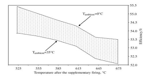
To, reiterate in a nutshell, it can be seen that: ambient temperature has a notable effect upon the power generated by the gas turbines, the rise in temperature after supplementary heating reduces thermal efficiency. However, megawatts of power generated goes up. Using both factors of supplementary firing and ambient temperature side by side can result in 170 MW of additional power generation, with the thermal efficiency downfall of 3-4%.
