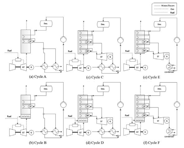
factor and R1-energy efficiency. The study considers three different types of combined cycle power plants, each of which is considered twice as with and without supplementary firing.
