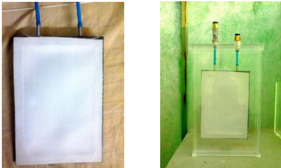
Figure 3.2 Membrane bio-tank and module
