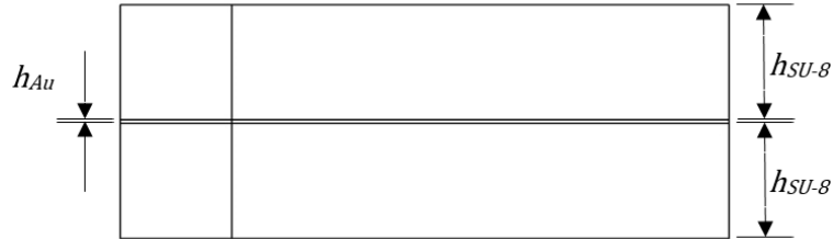
Figure 3.3: Cross-section of actuator with annotations
