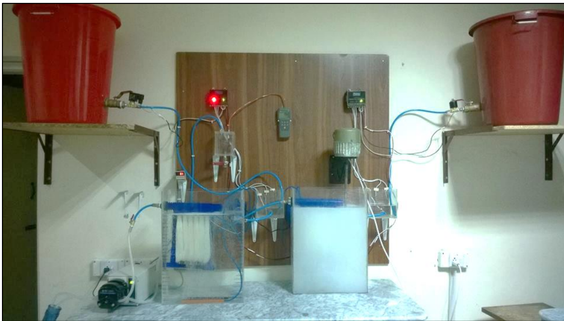
Figure 3.2: Installation of Submerged MBR
