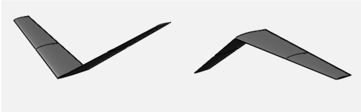
Figure 1.8: (a) Left: A V-tail setup with dihedral angle (b) Right: An inverted V-tail setup with anhedral angle.
