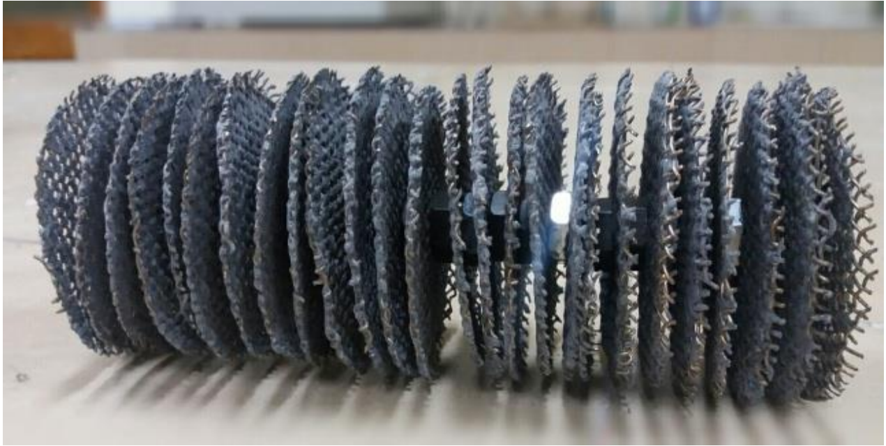
Fig.3.3. Pieces of wire mesh arranged on screw bar
