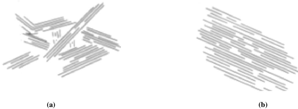
Fig. 2.4- Distribution of rod-like aramid structure in diluted solvent, (a) in liquid crystalline arrays, (b) nematic state for one array
