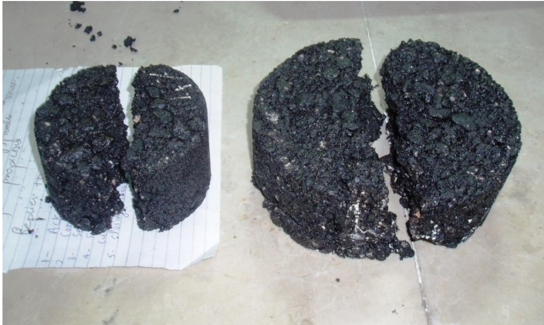
Figure 3.12: Failure of Specimens during Indirect Tension Test
