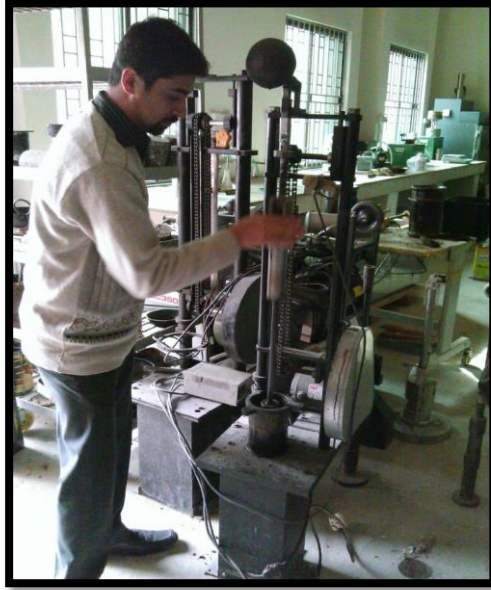
Figure 3.4: Compaction of Specimens by Compaction Pedestal
