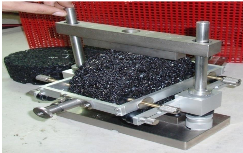
Figure 3.14: Jig Setup for Resilient Modulus Test
