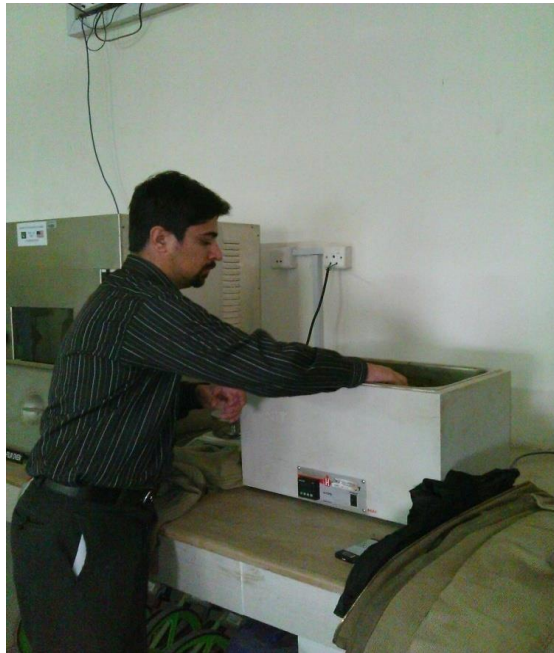
Figure 3.9: Specimen being put in Water bath for Conditioning
