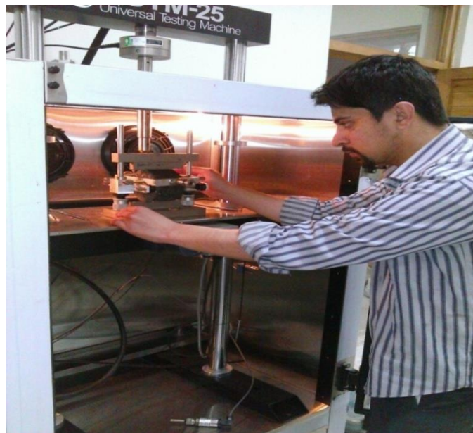
Figure 3.15: LVDTs Setup in UTM for Resilient Modulus Test
