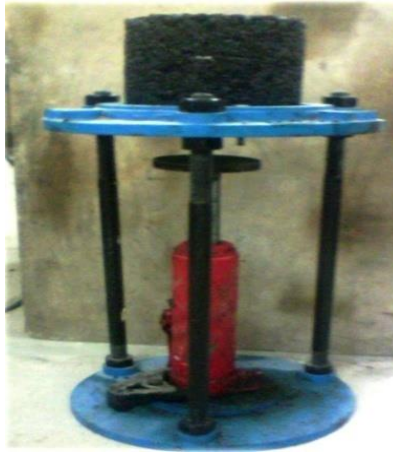
Figure 3.5: Extracting Jack for Extraction of Specimens
