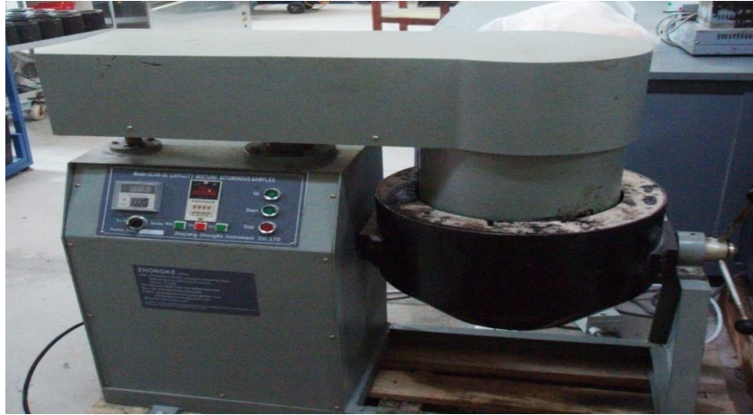
Figure 3.3: Mixing of Aggregates and Bitumen in Mechanical Mixing Machine
