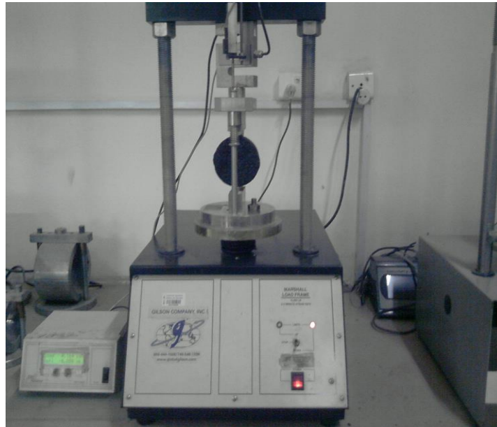
Figure 3.10 Splitting Tensile Test Set up
