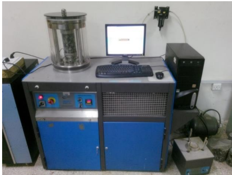
Figure 3.7 Asphalt mixture performance tester.
