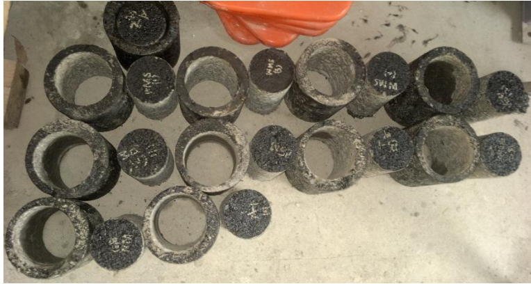
Figure 3. 5 Gyratory prepared specimen cored with waste rings.
