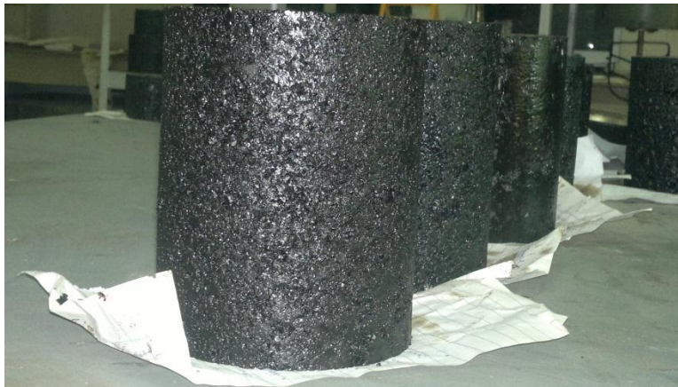
Figure 3.4 Specimen prepared from Gyratory compactor
