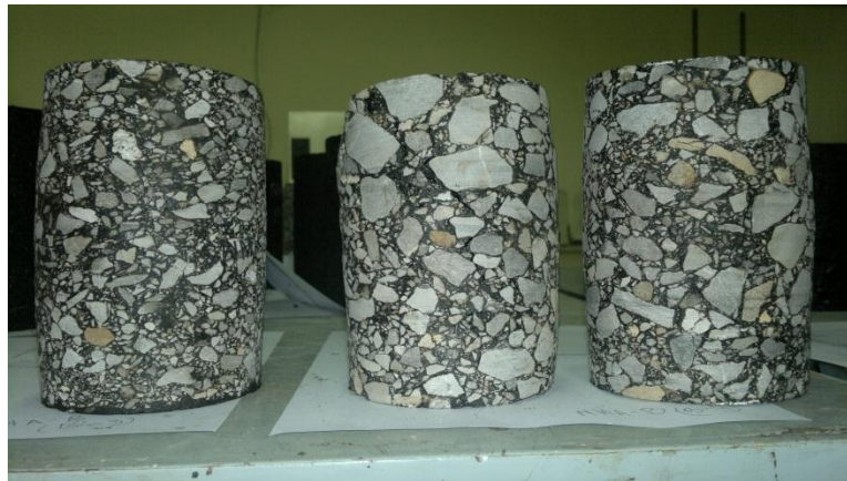
Figure 3. 8 Condition of samples after successful completion of FN test
