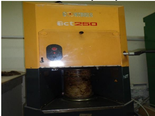
Figure 3.8: Gyratory Mold Placed in SGC
