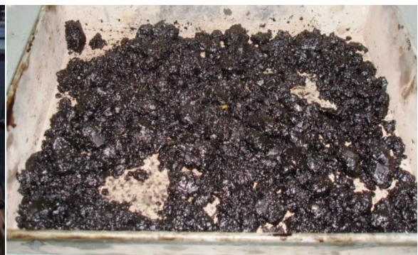
Figure 3.5: Mix Placed in Tray for Conditioning
