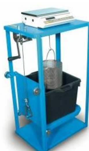
Figure 3.10: Theoretical Maximum Specific gravity and Bulk Specific gravity Apparatus
