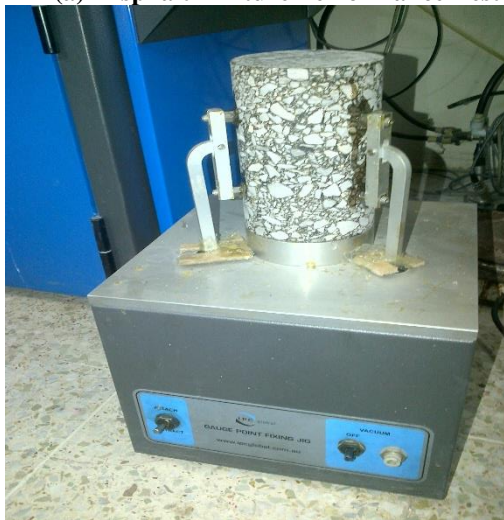
(b) Fixing Studs
