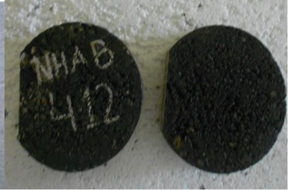
Figure 3.13: Saw Cut Specimens for Wheel tracker
