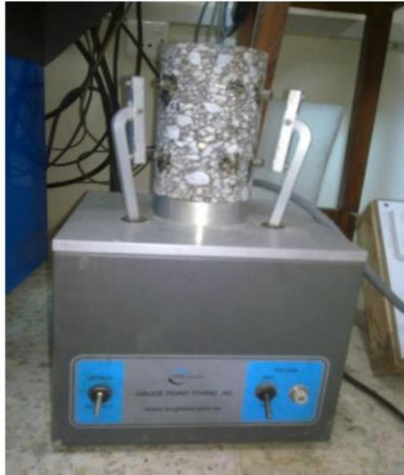
Figure 3.15: Studs fixing using gauge point fixing device
