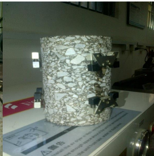
(c) Attaching LVDT Clamps
