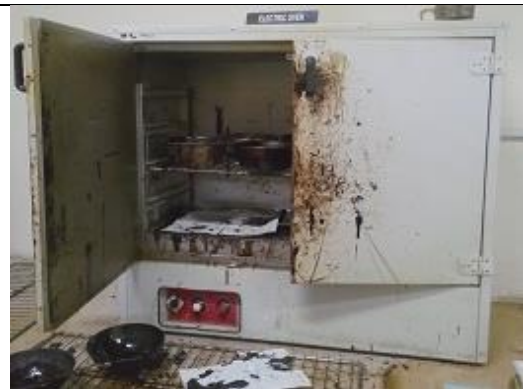
(b) Heating Asphalt prior to Mixing
