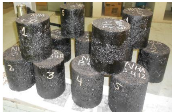
Figure 3.11: Gyratory Compacted HMA Specimens
