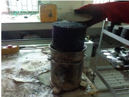
Figure 3.9: Extraction of Compacted Specimen
