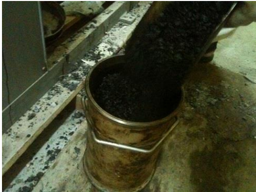
Figure 3.6: Transferring Conditioned Mixture in Preheated Gyratory Mold
