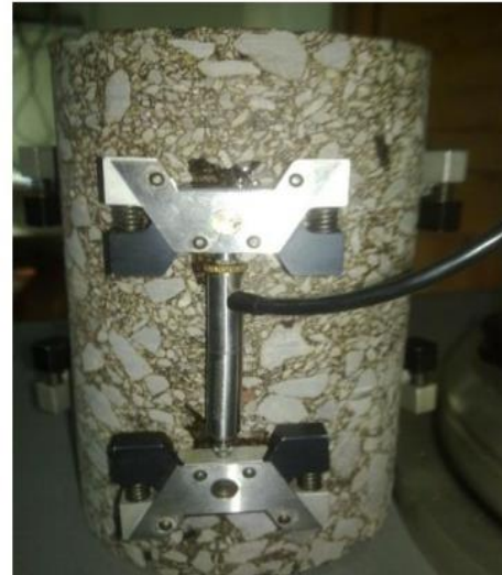
Figure 3.16: Clamps and LVDT's mounted on the sample
