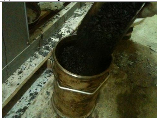
(g) Transferring Conditioned Mixture in Preheated Gyratory Mold
