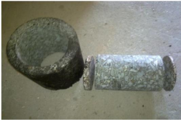
Figure 3.12: Cored and Trimmed Specimens with Waste ring
