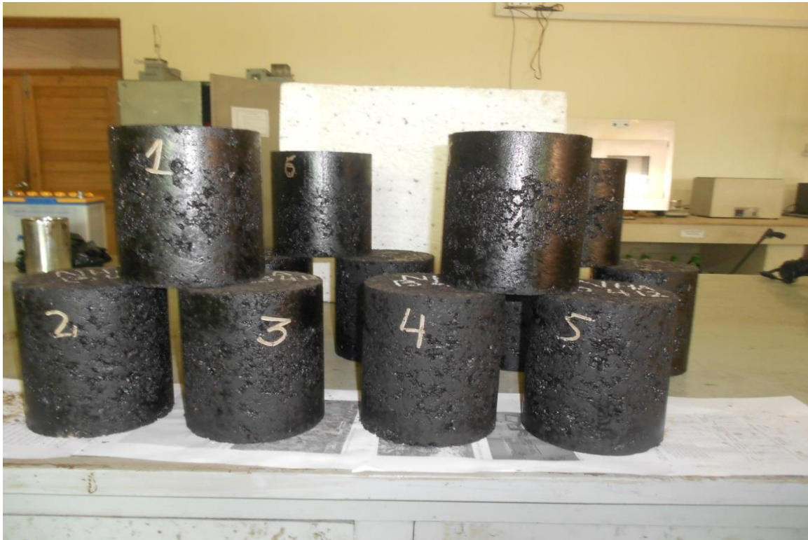
Figure 3.4 Specimens prepared using gyratory compactor
