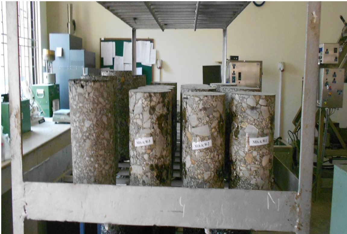
Figure 3.6 Specimens gathered in laboratory for dynamic modulus test
