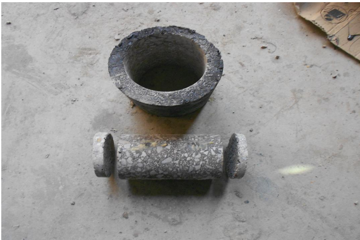
Figure 3.5 Cored and trimmed specimen alongwith waster rings.
