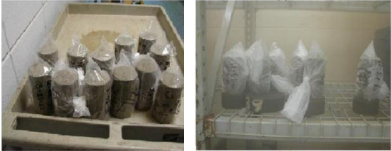
Figure 3.13: Curing of soil cement mixtures
