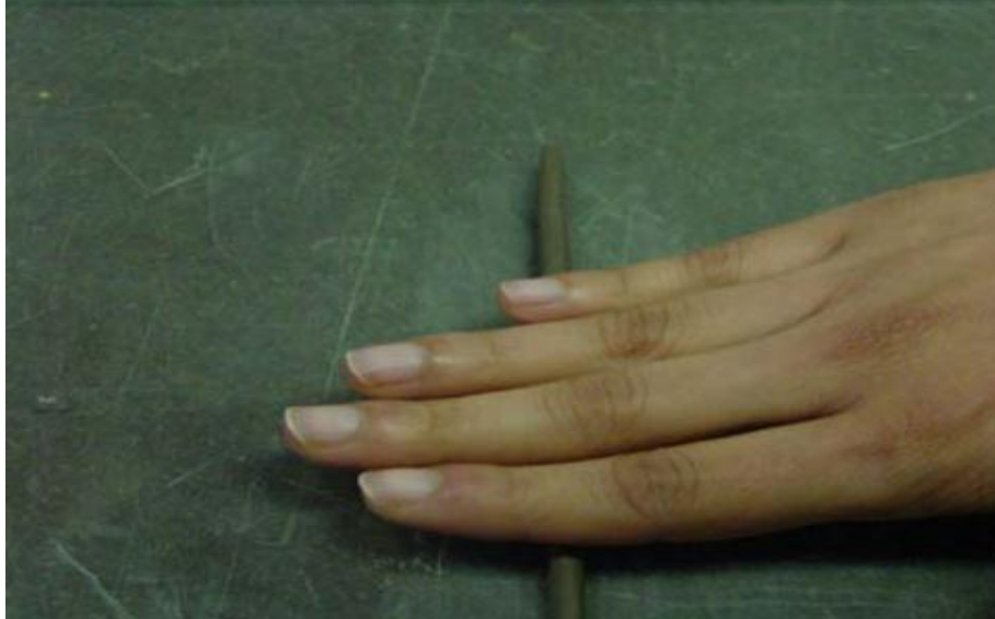
Figure 3.6: Sample preparation for Plastic limit
