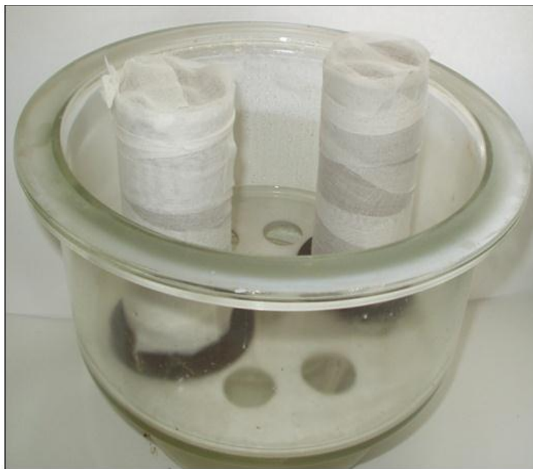
Figure 3.12: Soil lime mixture soaking
