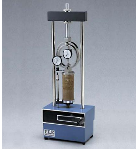
Figure 2.7: UCS testing equipment
