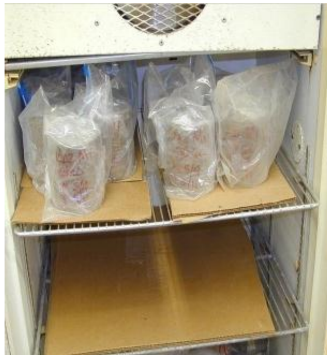
Figure 3.11: Curing modified specimen of lime
