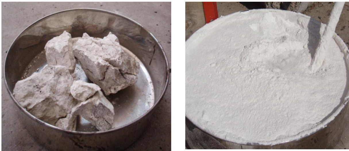
Figure 3.7: Hydrated lime Prepared in laboratory
