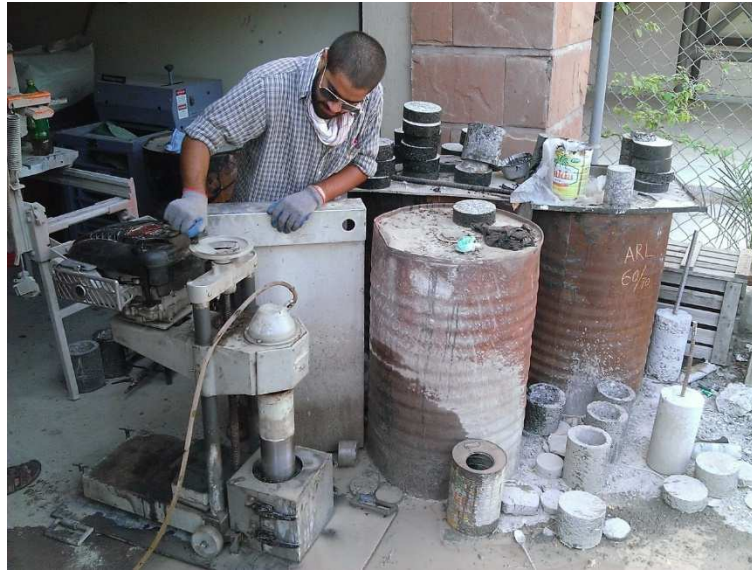
Figure 3. 5 Core cutting machine
