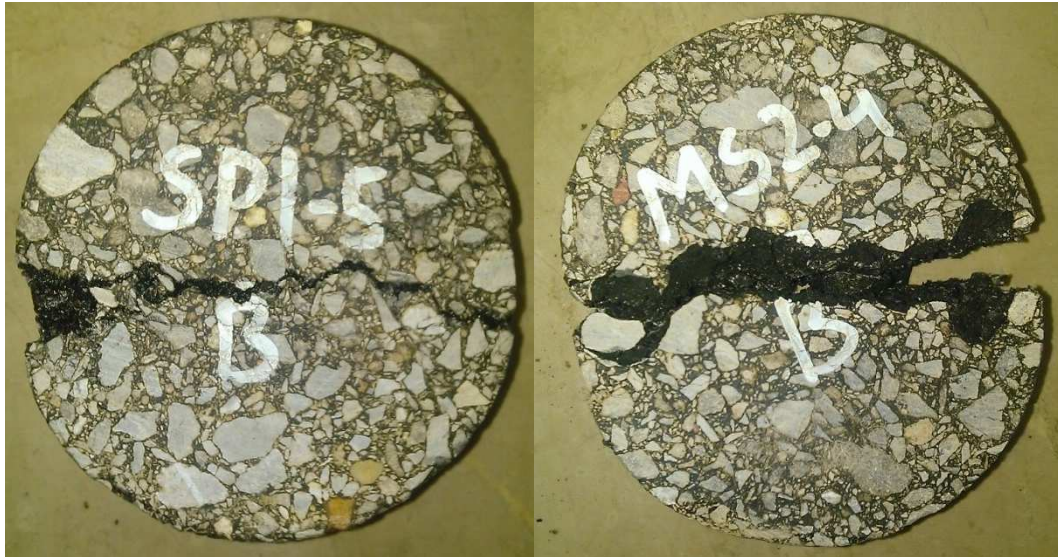
Figure 3. 8 Fractured samples due to repeated load applied
