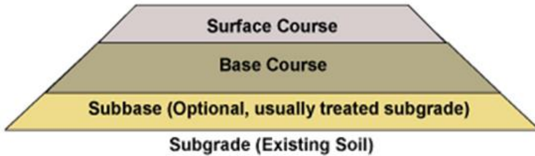
Figure 2.1: Pavement Structural Layers
