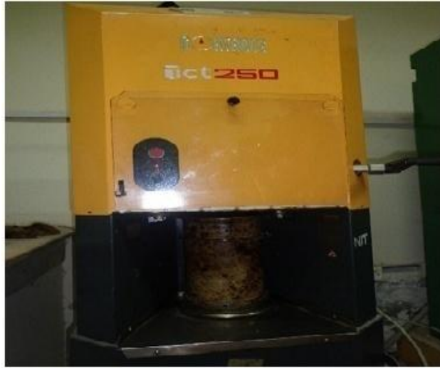
Figure 3.8: Gyratory Mold Placed in SGC
