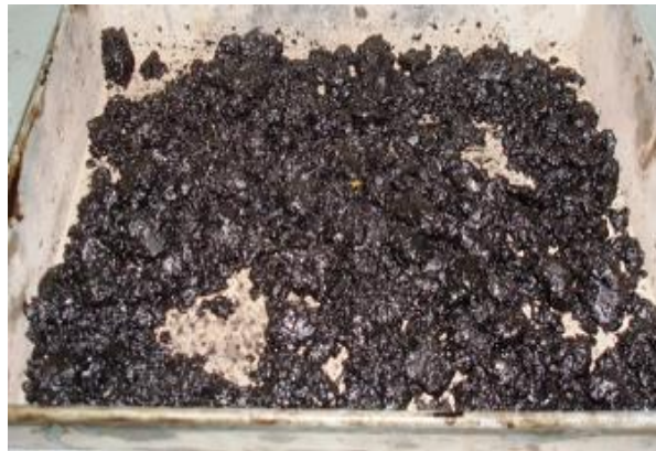
Figure 3.5: Loose Mix Placed in Tray for Conditioning
