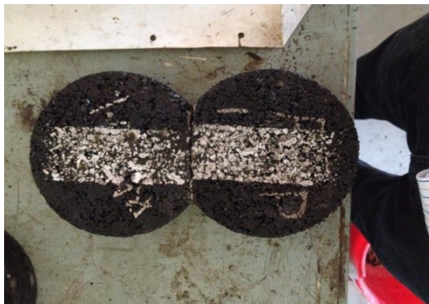
Figure 3.15: Saw cut specimens for wheel tracker test
