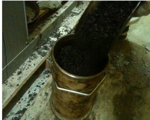
Figure 3.6: Transferring Conditioned Mixture in Preheated Gyratory Mold
