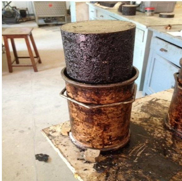
Figure 3.9: Extraction of Compacted Specimen
