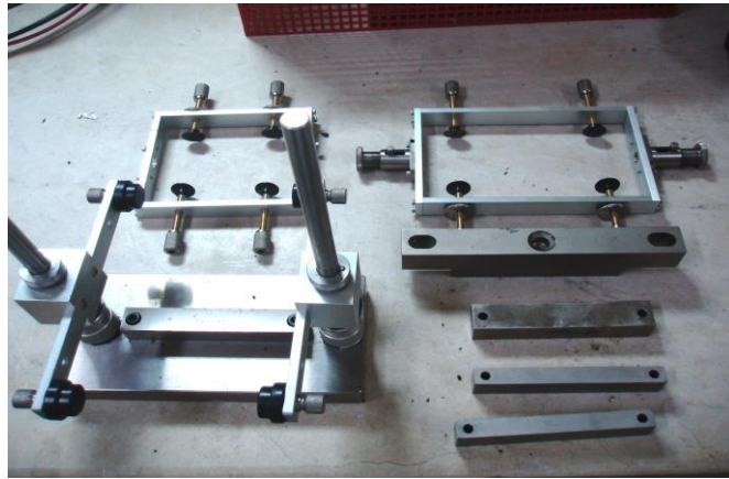
Figure 3.29: Specimen Jig Accessories for Resilient Modulus Test
