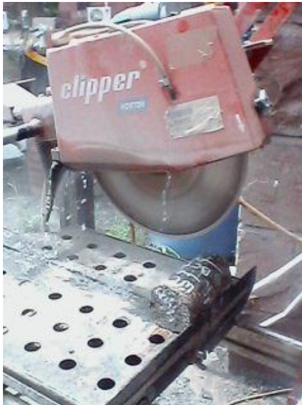
Figure 3.11: Saw Cutting of Samples
