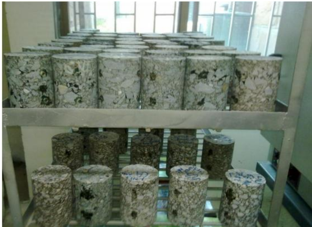
Figure 4.14: Cored and Trimmed Specimens ready for Testing
