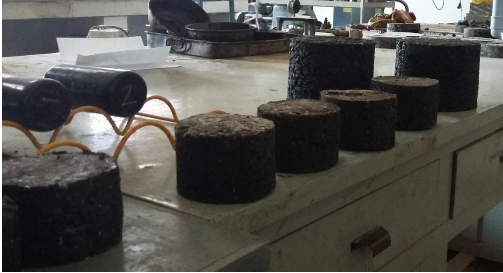
Figure 4.3: Samples Prepared for Wearing and Base Course OBC
