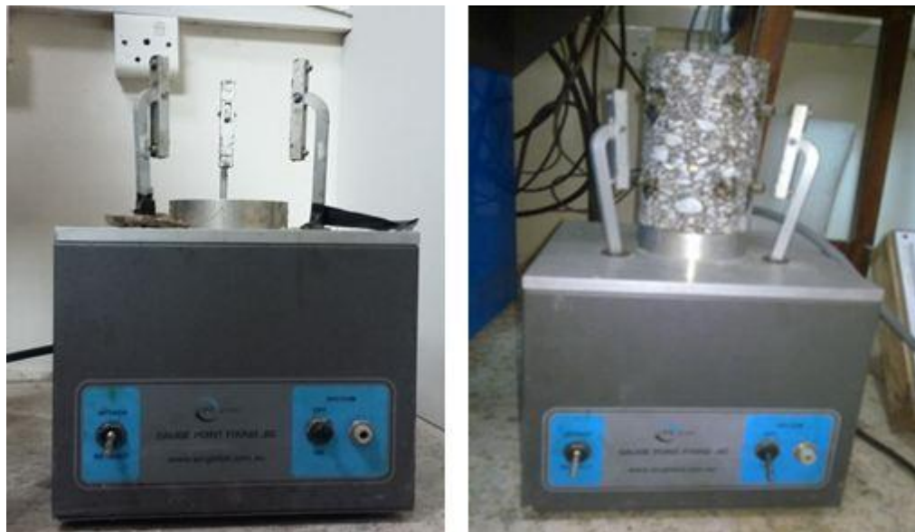
Figure 4.15: Stud Fixing Machine without and with Sample
