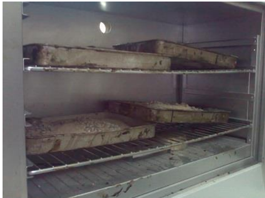
(a) Heating Aggregates Prior to Mixing
