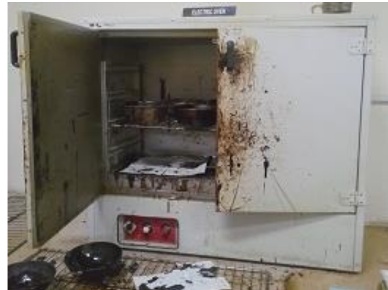
Figure 3.4: Heating Bitumen Binder Before Mixing
