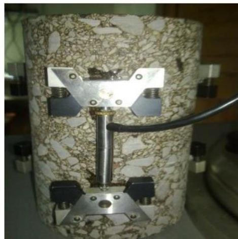
Figure 3.21: LVDT's Attached Sample
