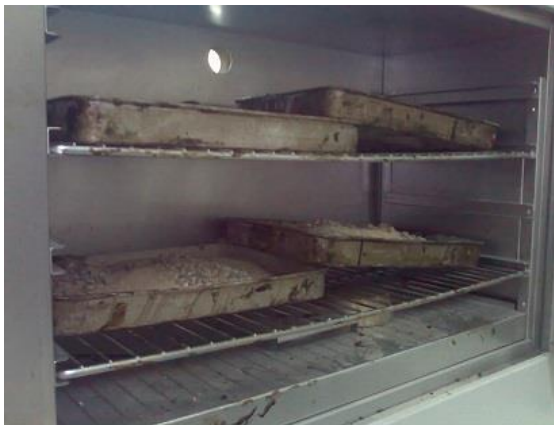
Figure 3.3: Heating Aggregates Before Mixing
