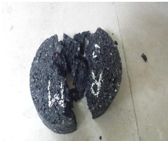
Figure 3.16: Failed Samples during IDT Test
