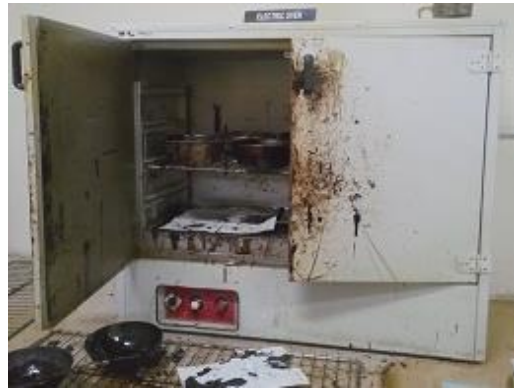
(b) Heating Asphalt prior to Mixing
