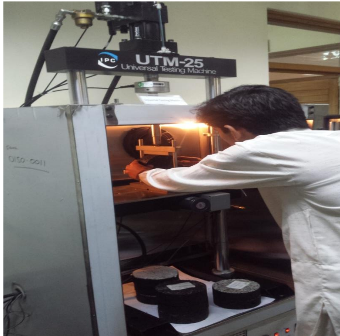
Figure 3.19: LVDTs Setup in UTM for Resilient Modulus Test
