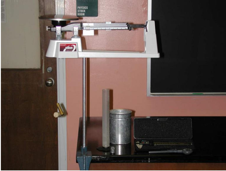
Figure: 4.6: Apparatus used for measuring Density by Archimede's Method
