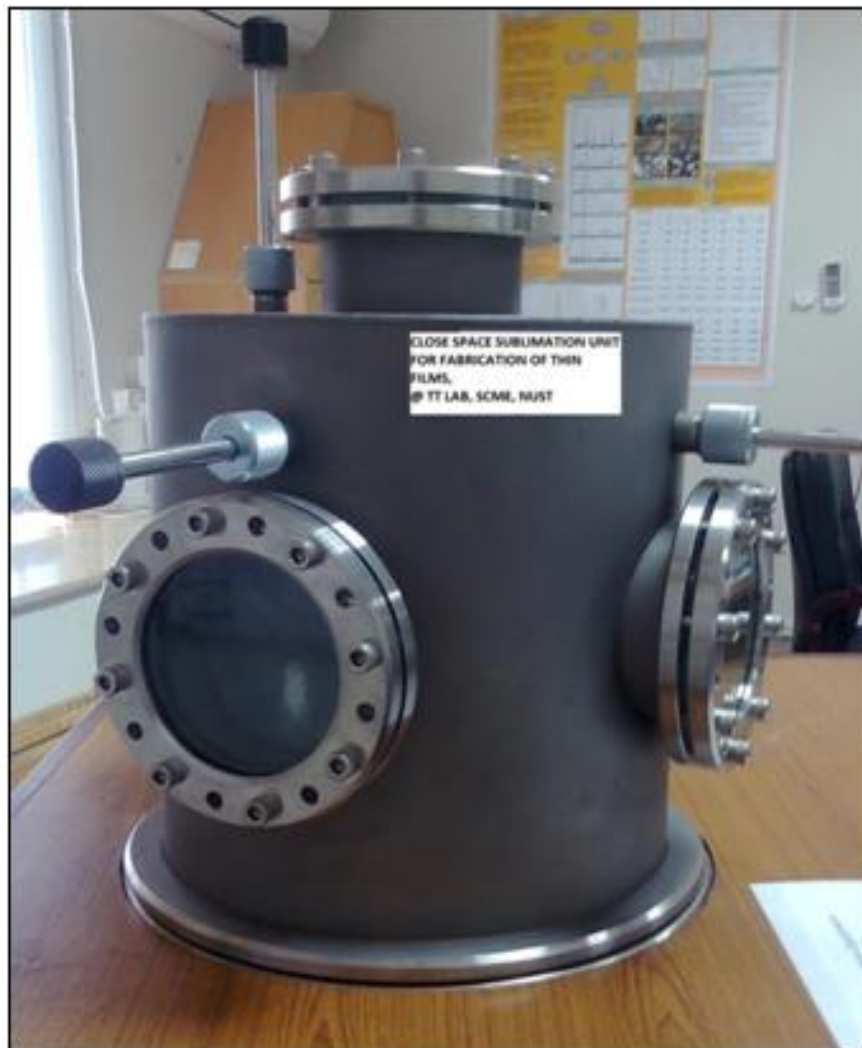
Figure 5.1: Photo of the CSS equipment built in this project
