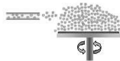
Fig. 4.3: Spray coating process [35]
