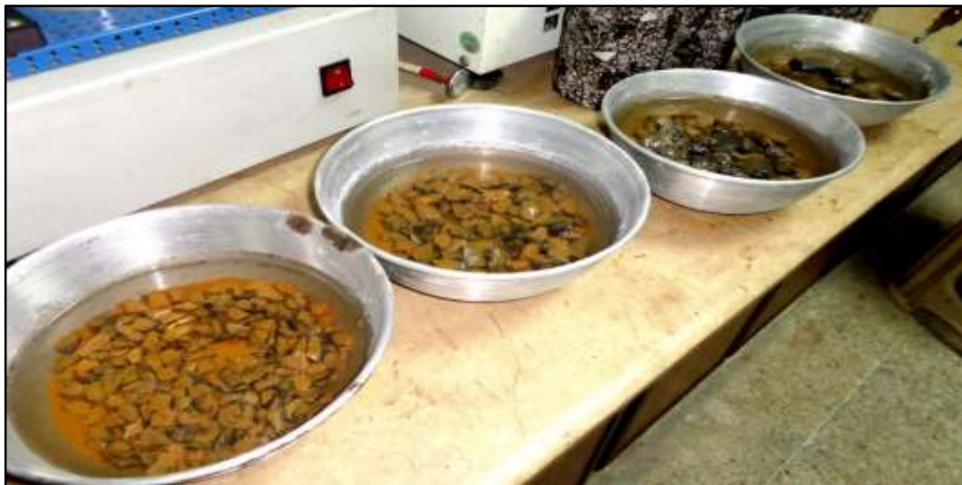
Figure 3.7: Water Absorption Test of Coarse Aggregate
