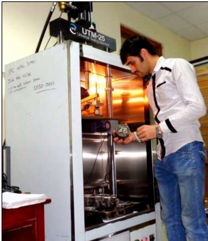
Figure 3.36: ITS Testing using UTM
