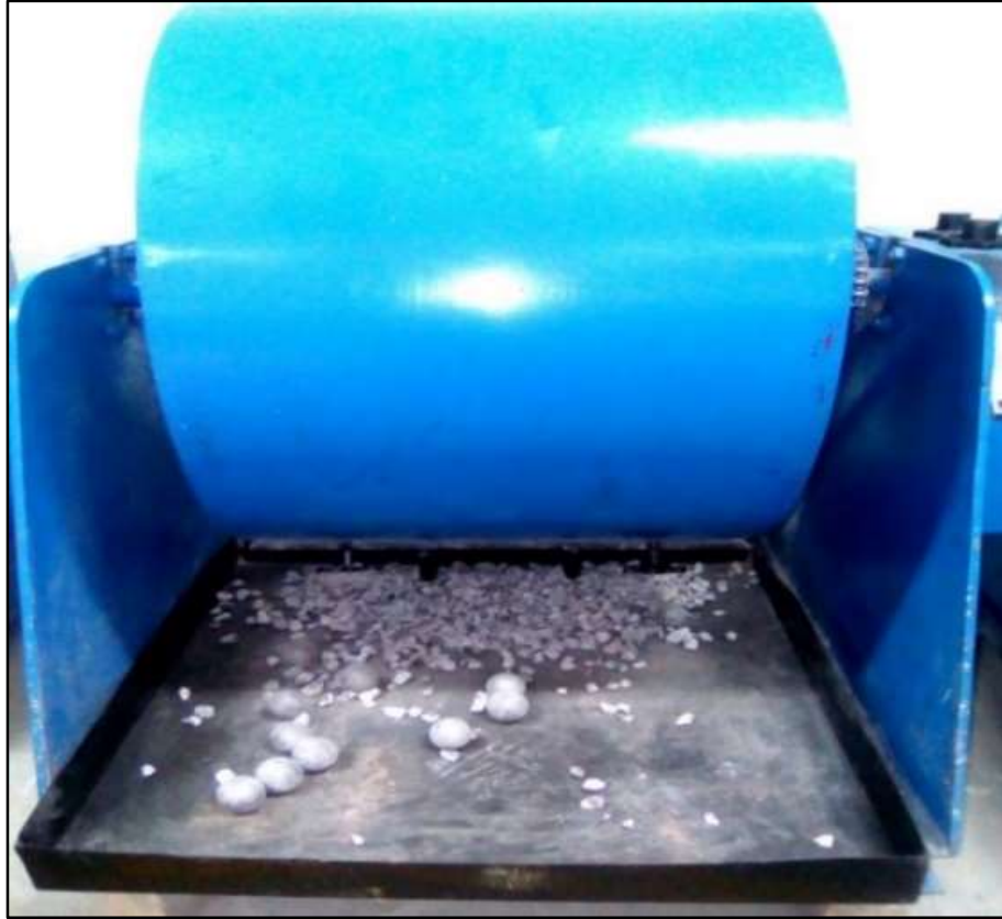
Figure 3.11: Los Angeles Abrasion Machine
