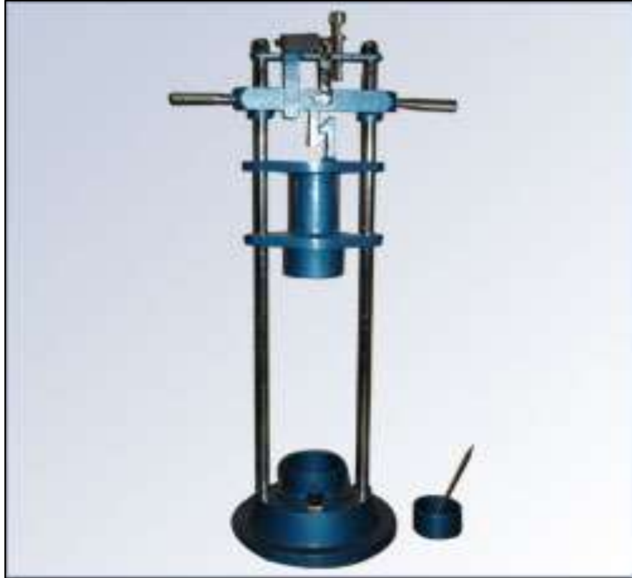
Figure 3.9: Crushing Value Test Apparatus
