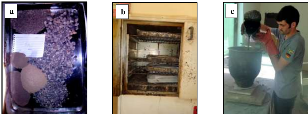
Figure 3.19: (a), (b) & (c): Preparation of Aggregates and Bitumen for Mix
