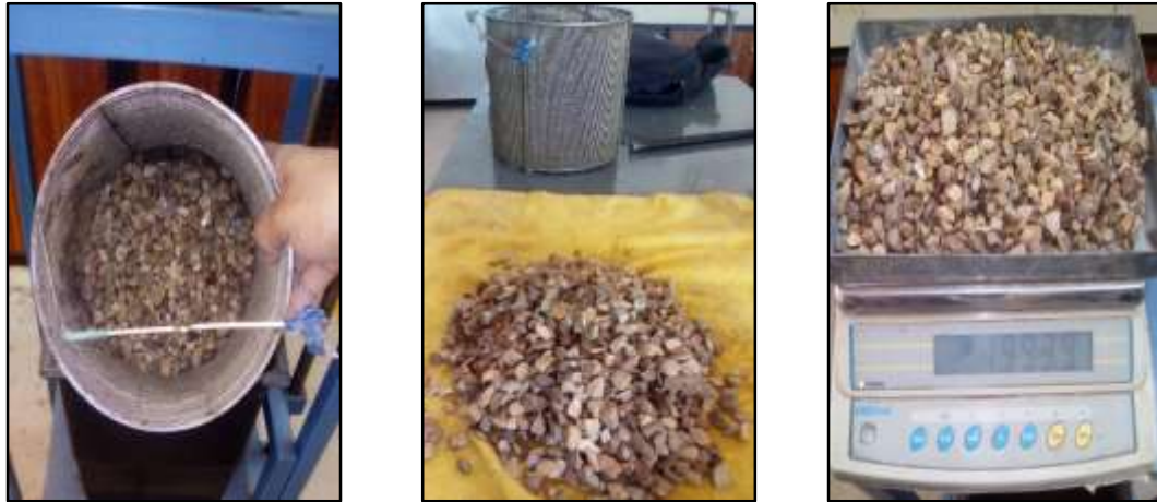
Figure 3.6: Specific Gravity Test of Coarse Aggregate
