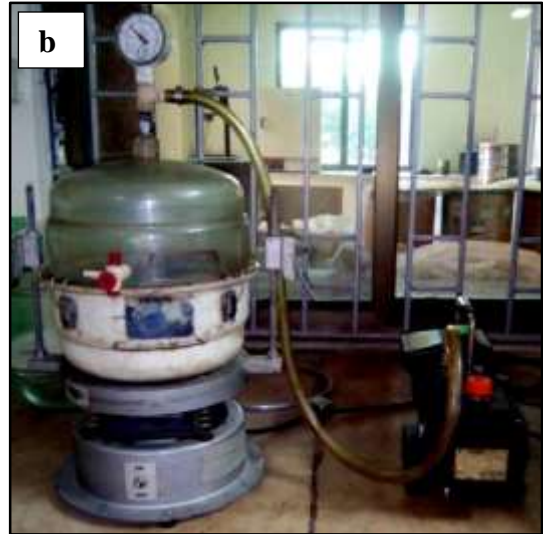
Figure 3.25: Gmm Calculation for Asphalt Mix
