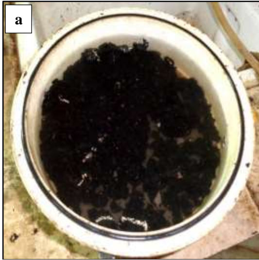
Figure 3.25: Gmm Calculation for Asphalt Mix
