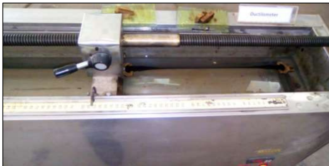
Figure 3.14: Ductility test of Bitumen
