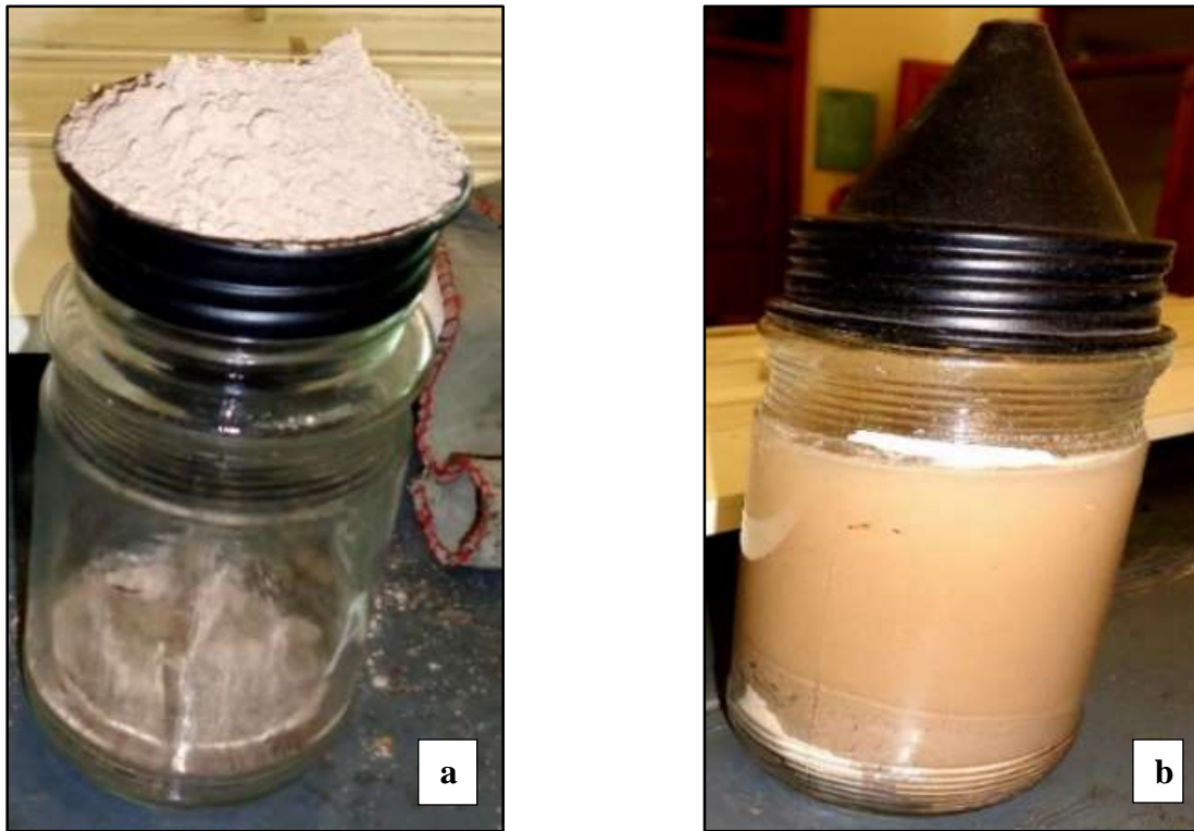
Figure 3.8 (a) & (b): Specific Gravity Test of Fine Aggregate (Filler)
