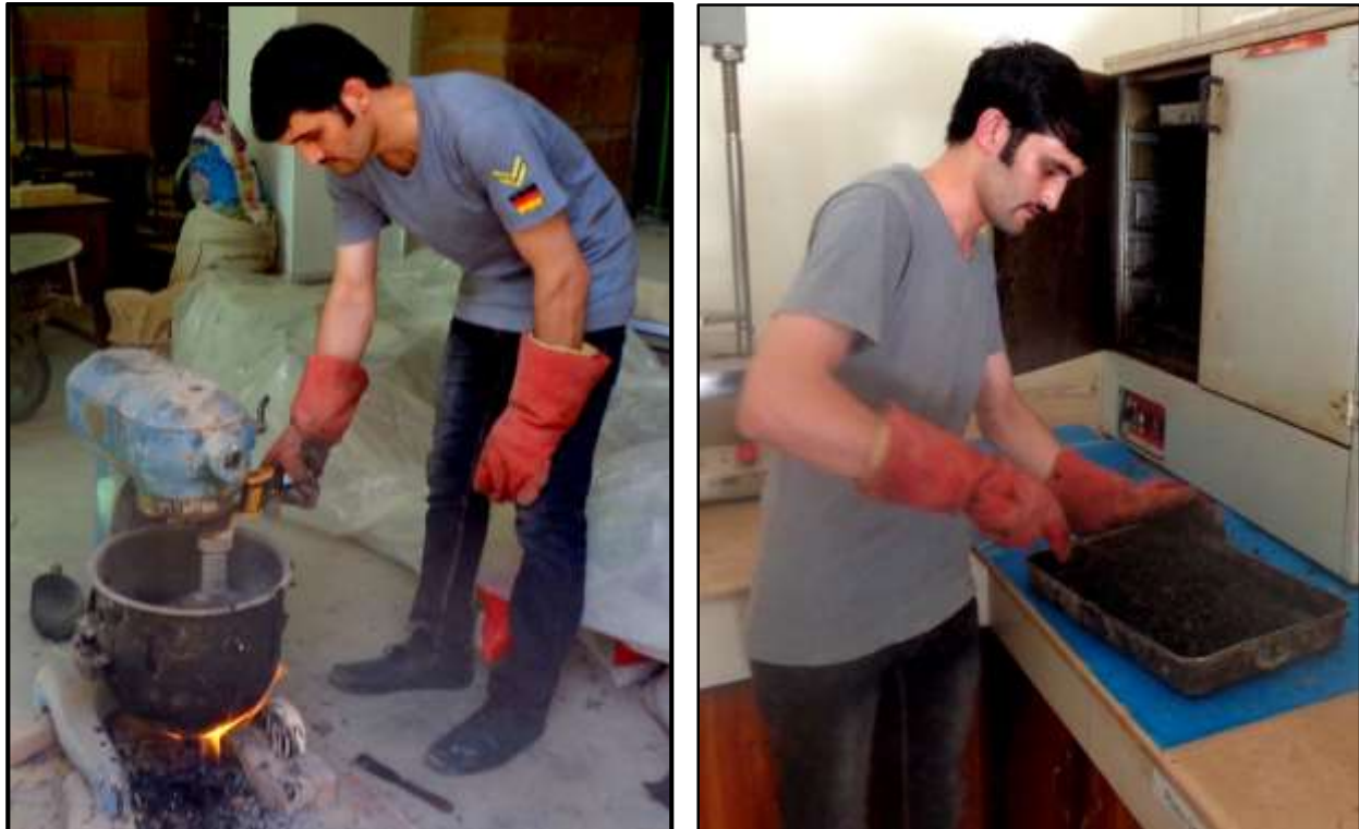
Figure 3.20: Asphalt Mixing and Conditioning
