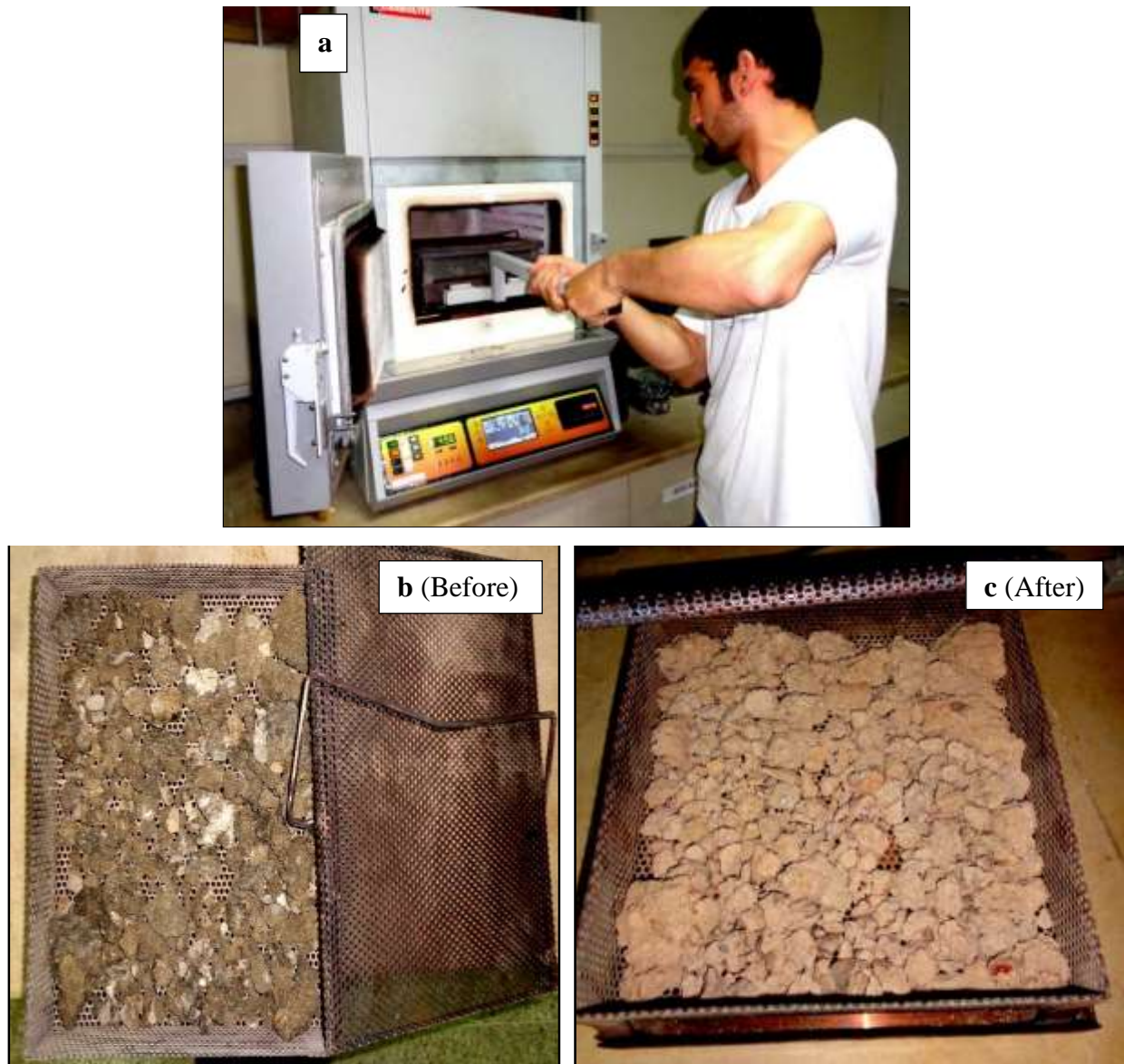
Figure 3.12: (a), (b) & (c): Determination of Asphalt content in RAP by Carbolite
