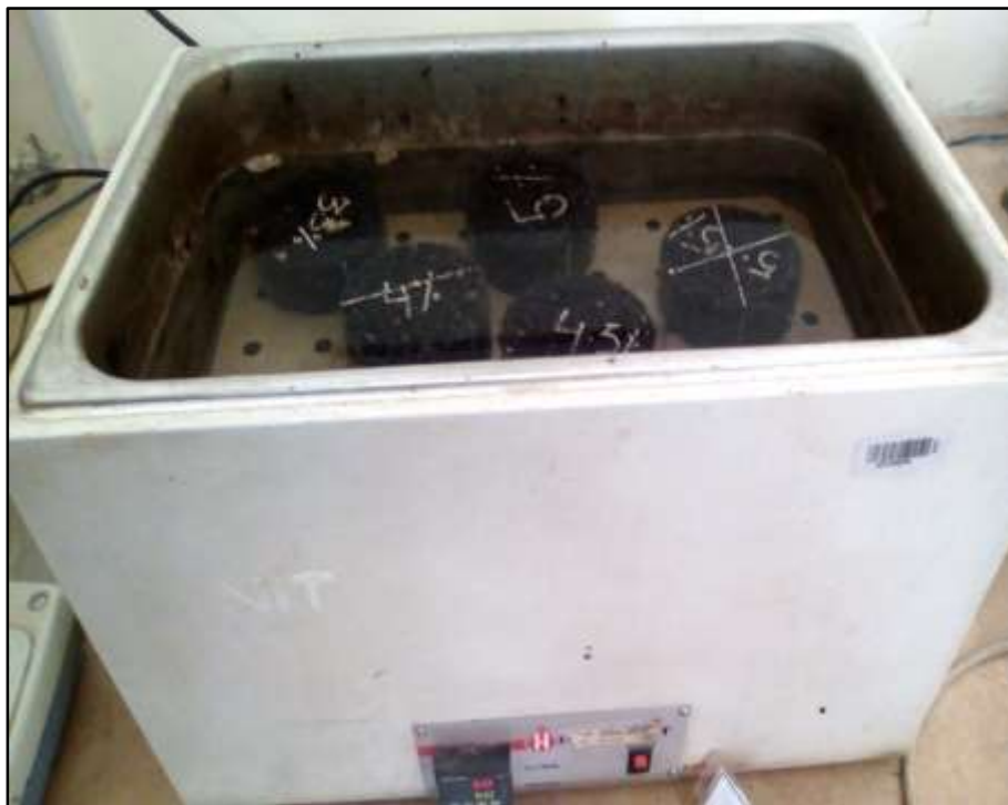
Figure 3.24: Marshal Samples Placed in Water Bath
