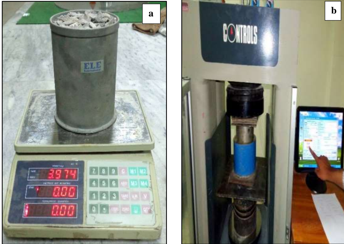
Figure 3.10 (a) & (b): Impact Value Test of Aggregate
