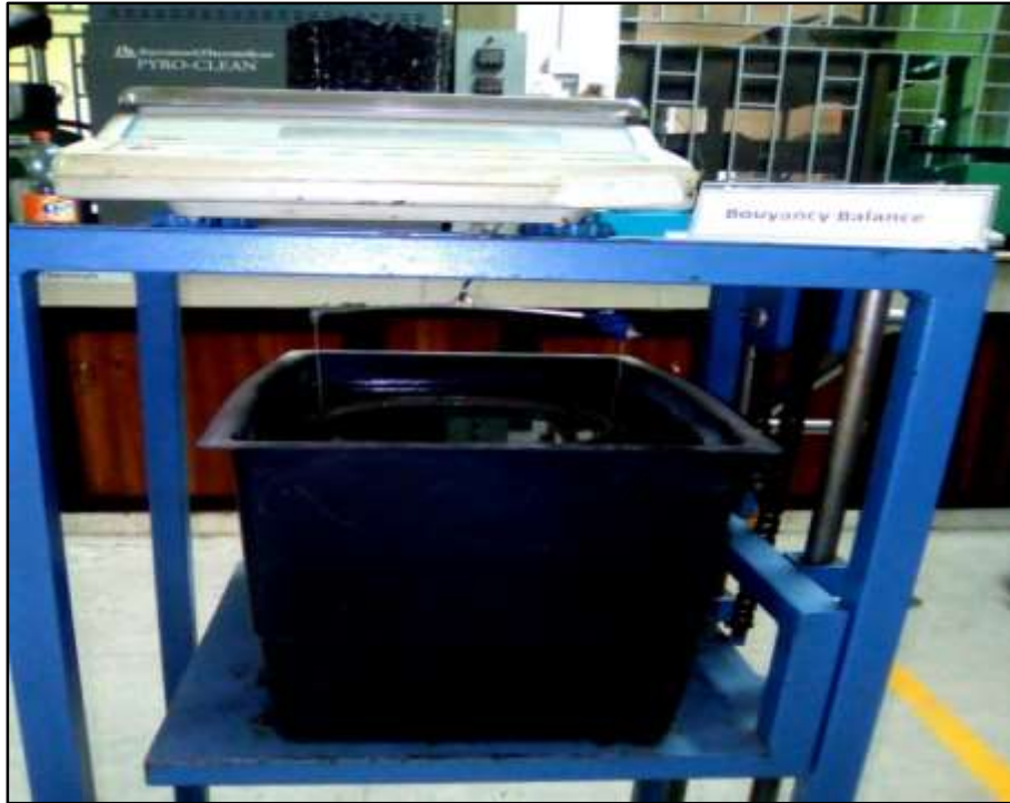
Figure 3.23: Gmb Calculation for Marshal Sample
