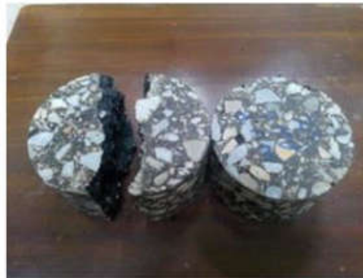
Figure 3-10: ITS Test sample before and after breakage
