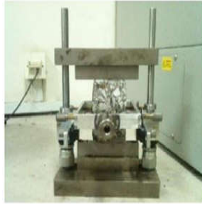
Figure 3-11: Sample in Jig Setup of UTM-25P
