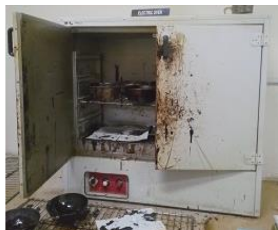
Figure 3.4: Heating Bitumen Binder Before Mixing
