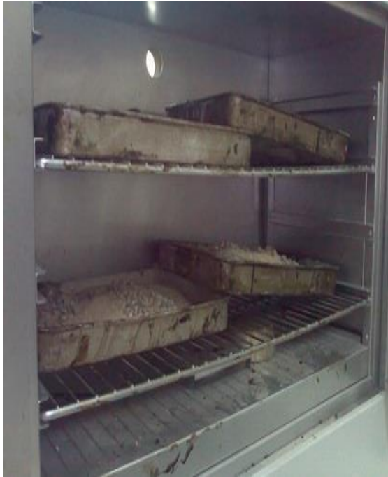
(a) Heating Aggregates
