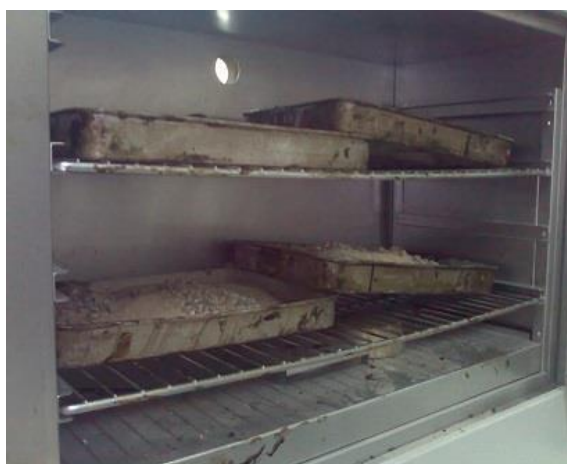
Figure 3.3: Heating Aggregates Before Mixing
