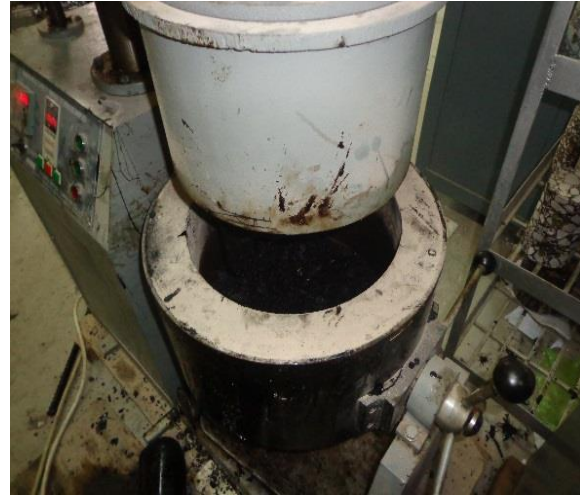
Figure 3.6: Mixing of Mixtures
