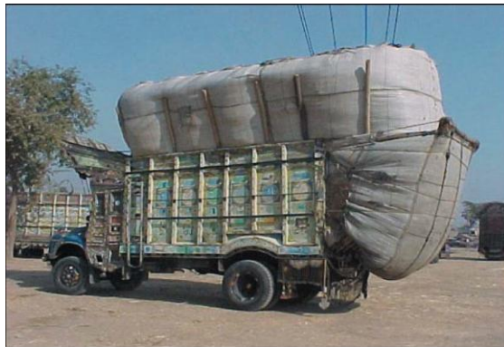
Figure 0.1 Excessive Axle Loads Due to Overloading
