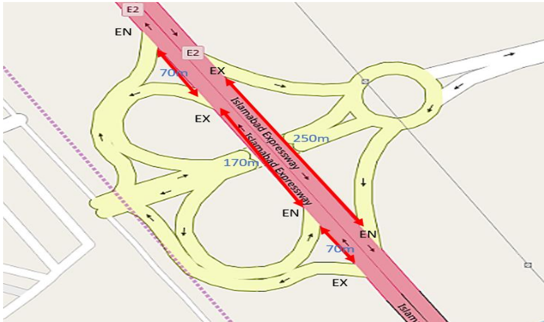
Figure 5.21: Gulberg distance between ramps
