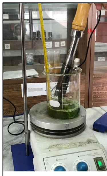
(b) Rod-type heater immersed in the boiling salt solution
