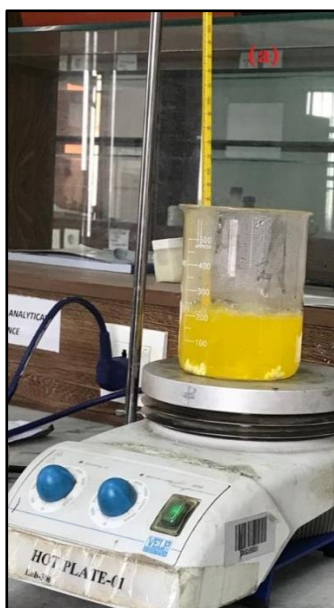
(a) Dissolution of precursor salts and citric acid in water
