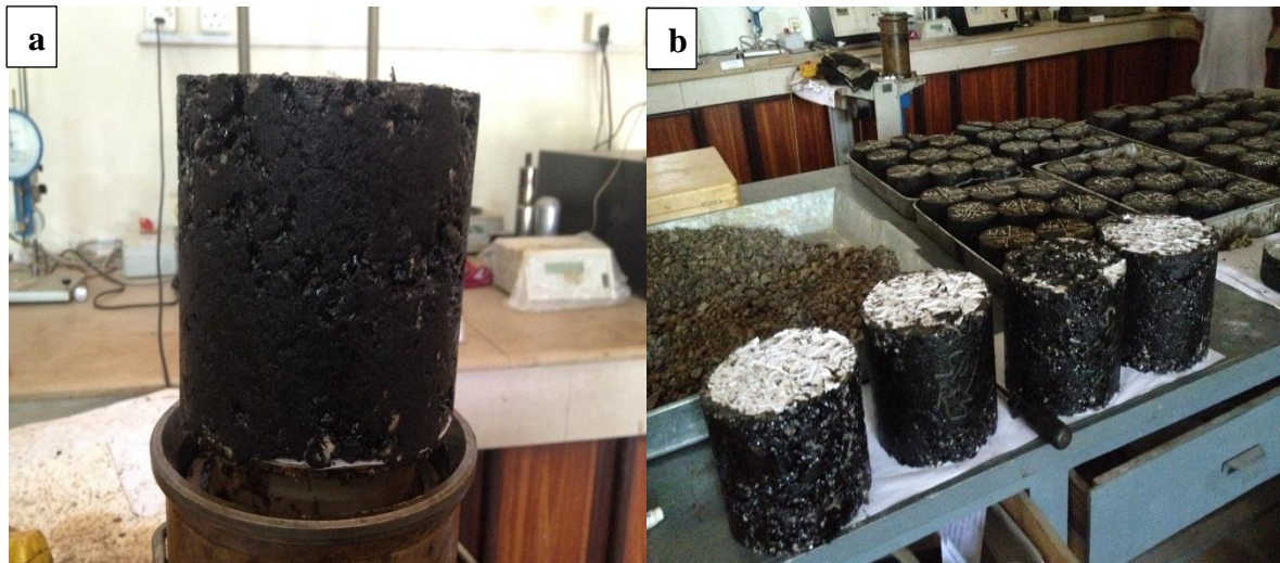
Figure 3.17: (a), (b) Gyrotory Compacted
