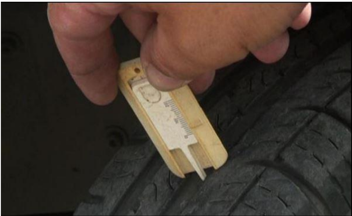
Figure 5. 3: Tyre Checking Procedure with Gauge.
