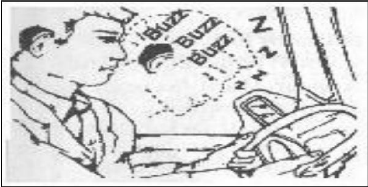
Figure 5. 2: Dozing Alert Alarm Mechanism –Buzzing on 15 Degree Head Bend..
