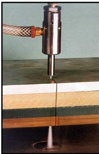
Abrasive Water Jet Cutting
