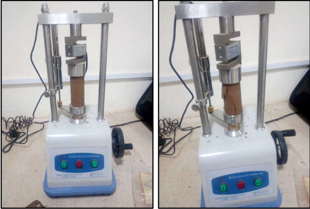
Figure 3-3 (a,b) UCS Testing of Natural Soil
