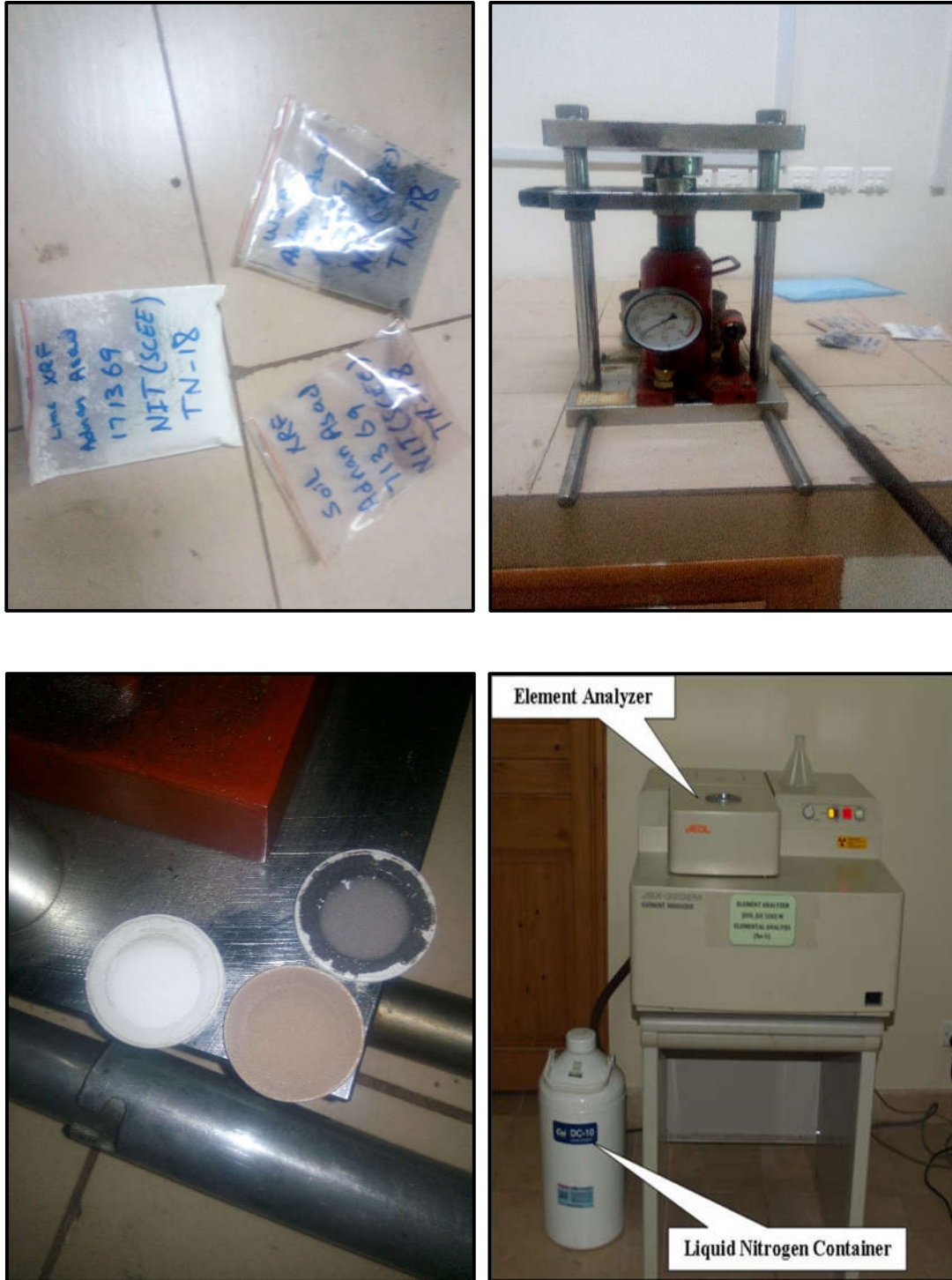
Figure 3-7 (a,b,c,d) Chemical Testing of Material Using XRF
