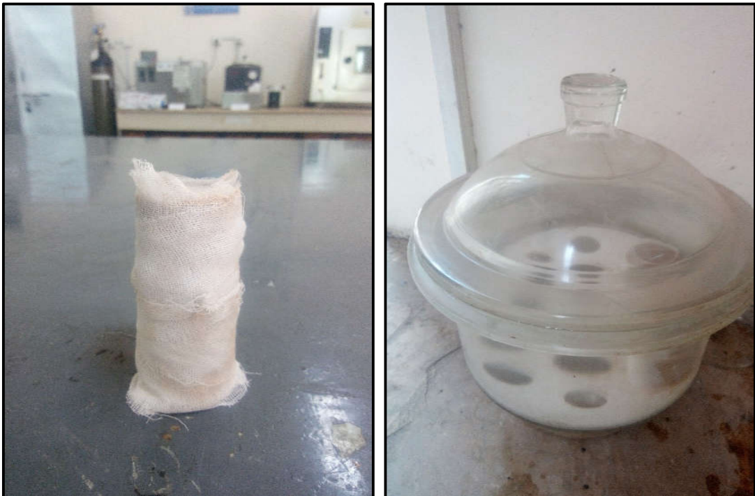
Figure 3-4 (a,b) Soaking of UCS Samples
