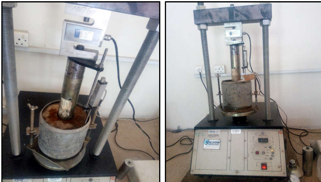
Figure 3-6 (a,b) CBR Testing
