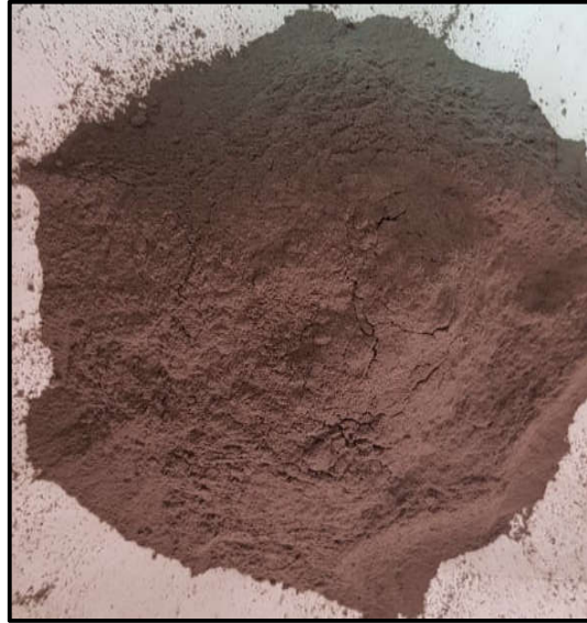
Figure 3-2 (b) WSA after Grinding
