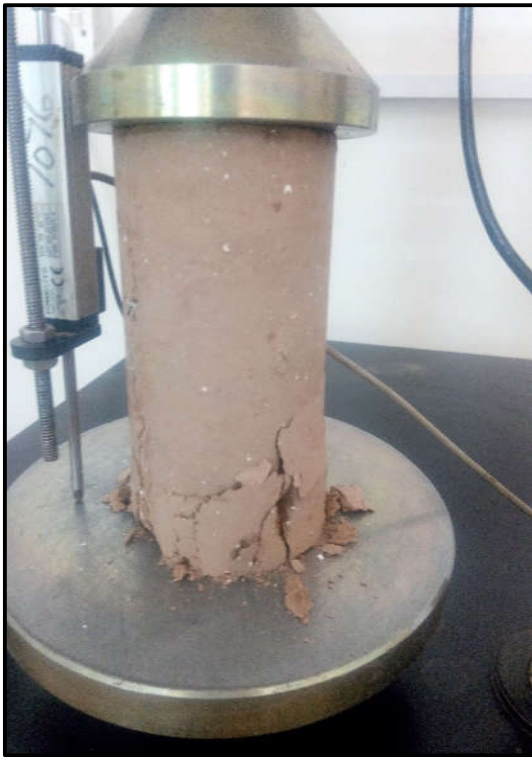
Figure 3-8 (a,b,c,d) UCS Testing Soil Lime Mix
