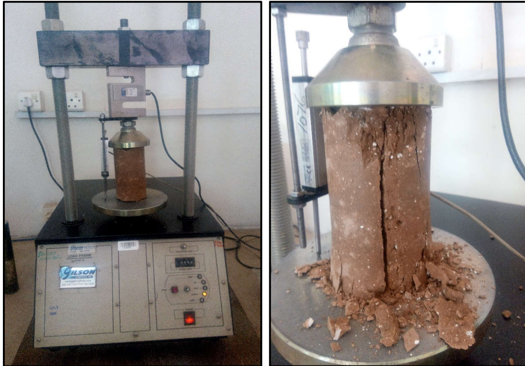
Figure 3-9 (a,b) UCS Testing Soil-Lime-WSA Mix
