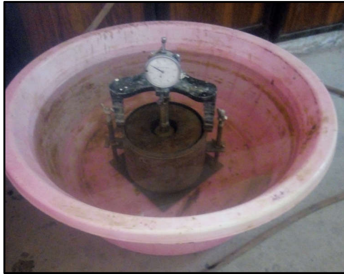
Figure 3-5 Soaking and Swell Measurement of CBR Sample
