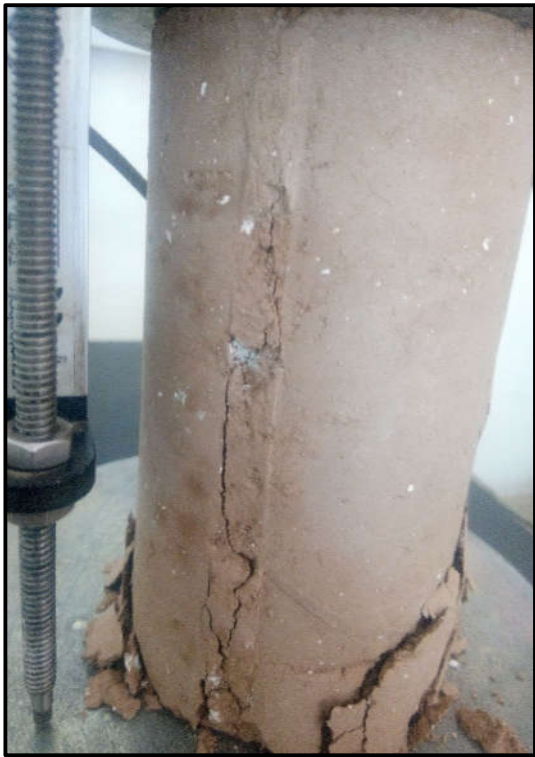
Figure 3-8 (a,b,c,d) UCS Testing Soil Lime Mix
