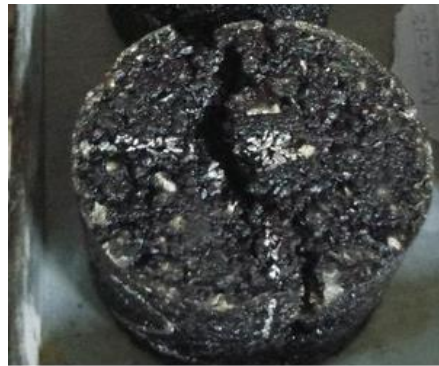
Figure 3. 13: Sample cracks under ITS test
