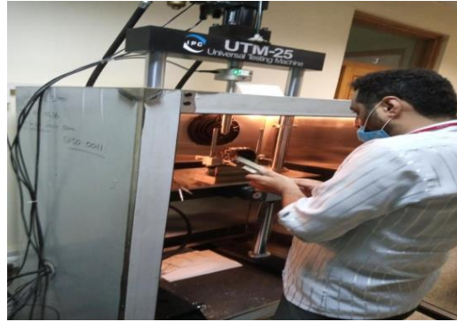
Figure 3. 14: Performing ITS test
