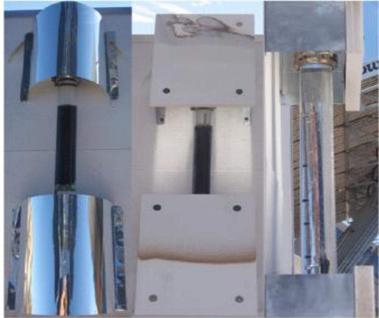
Figure 2-12: Liquid Immersion Concentrated Photovoltaic Module
