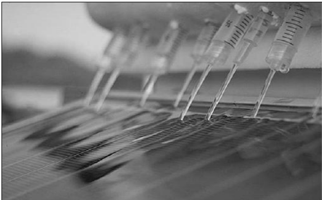
Figure 2-5: Water Flow Over the PV Modules by Nozzles
