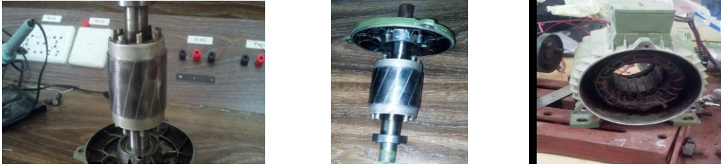
Fig. 4.3 Induction Motor's Rotor and Stator
