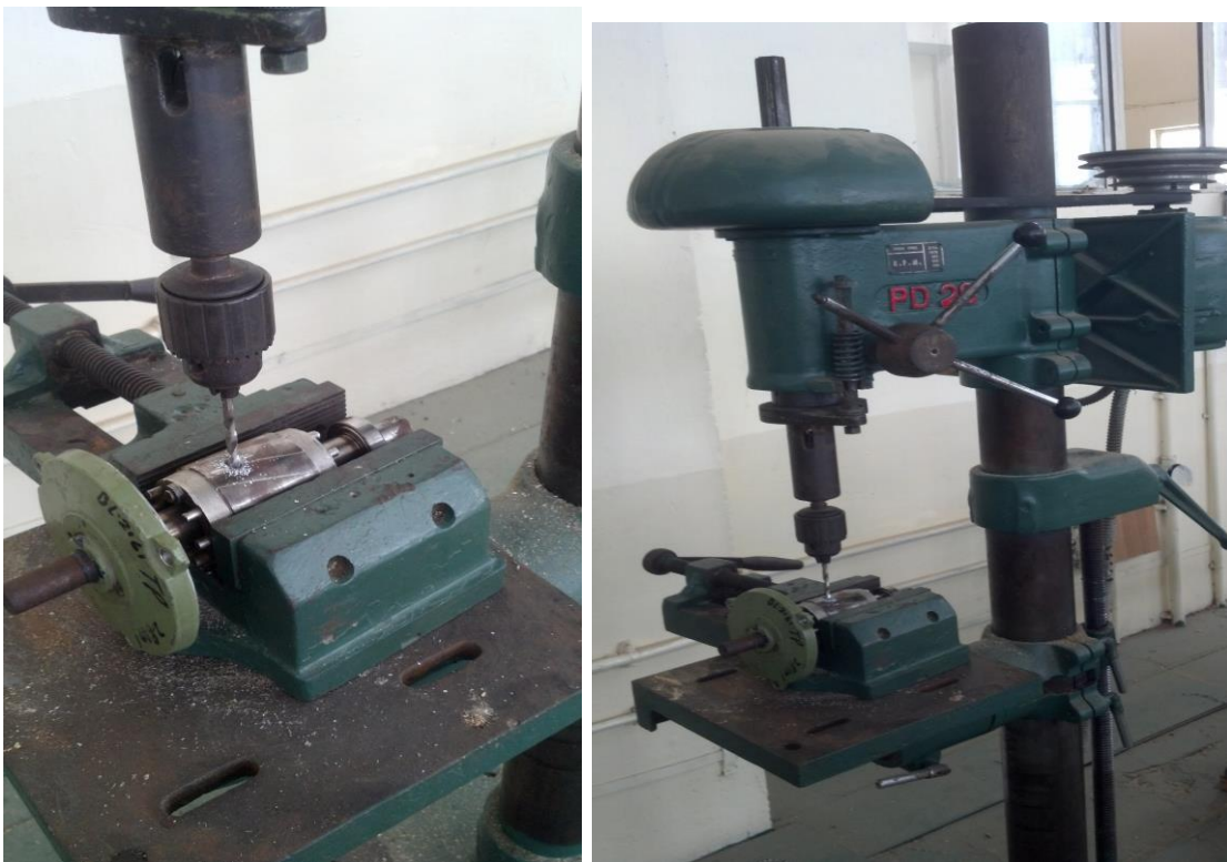
Fig. 4.5. Fault Injection by Mean of Drilling the Rotor Bar
