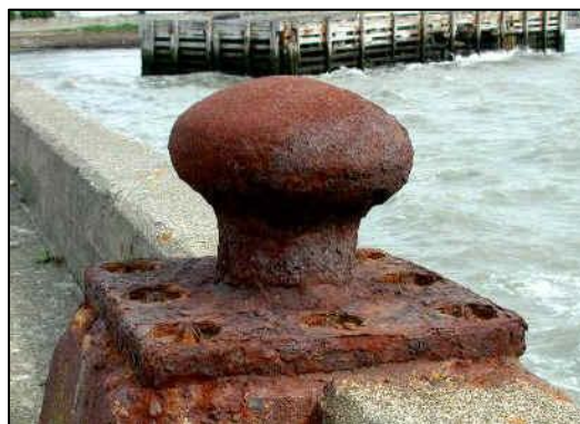
Figure 2-3; Uniformly corroded surface [15]
