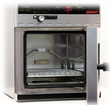
Step 5 Dried in vacuum oven at 40°C at 450mbar pressure
