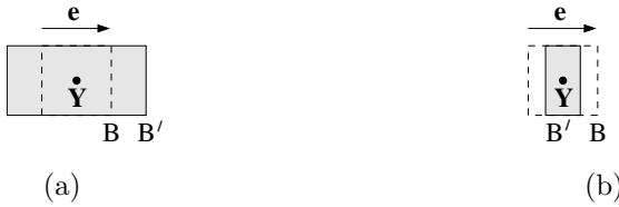
Fig. 4.5 Illustration of homogeneous extensions along a direction \mathbf{e} . (a) \lambda > 1 . (b) 0 < \lambda < 1 .
