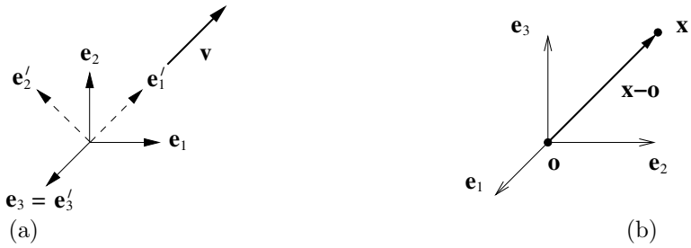
Fig. 1.3 Graphical illustration of orthonormal bases and a coordinate frame. (a) two orthonormal bases for \mathcal{V} . (b) Cartesian coordinate frame for \mathbf{E}^3 .
