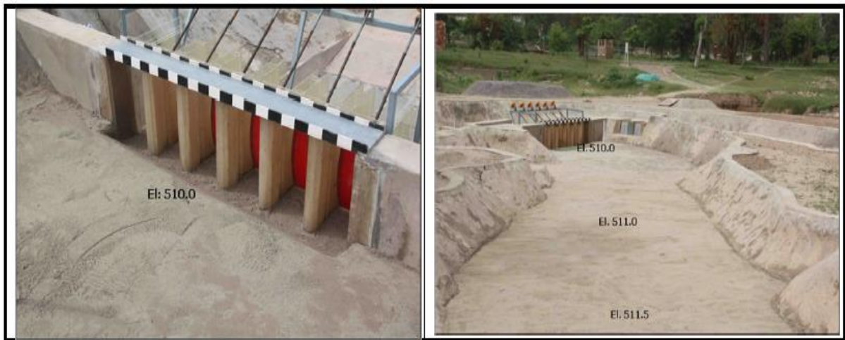
Figure 4.6: Sediment bed as moulded on model before test run
