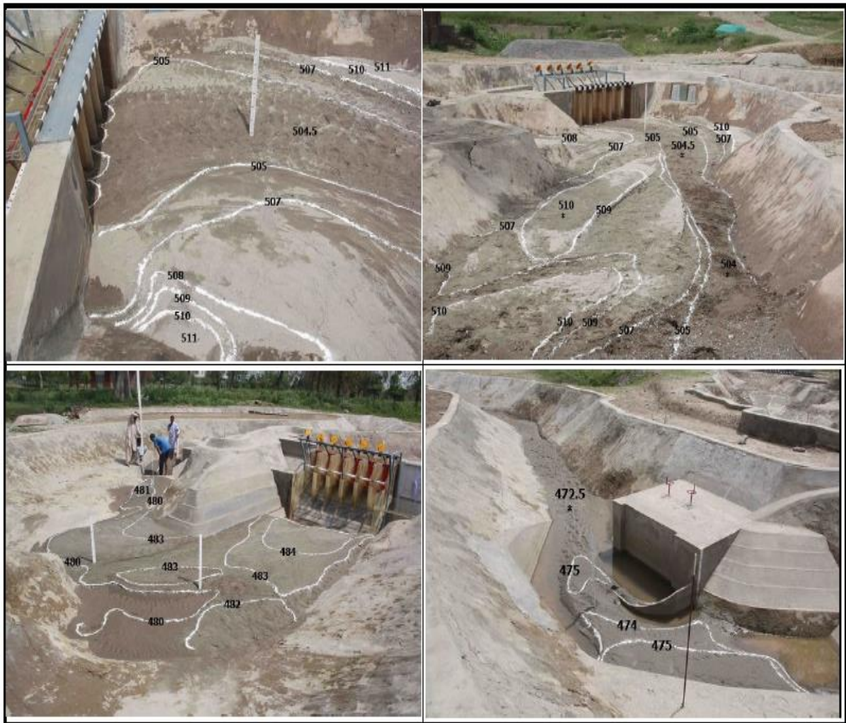
Figure 4.7: Case 1 – Flushing-affected area and sedimentation
