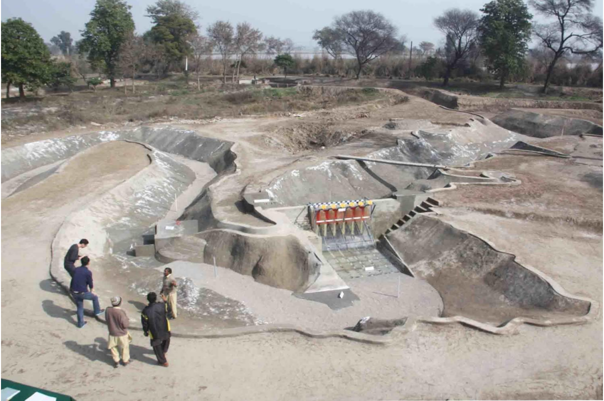
Figure 4.1: Model as constructed (scale 1:40)
