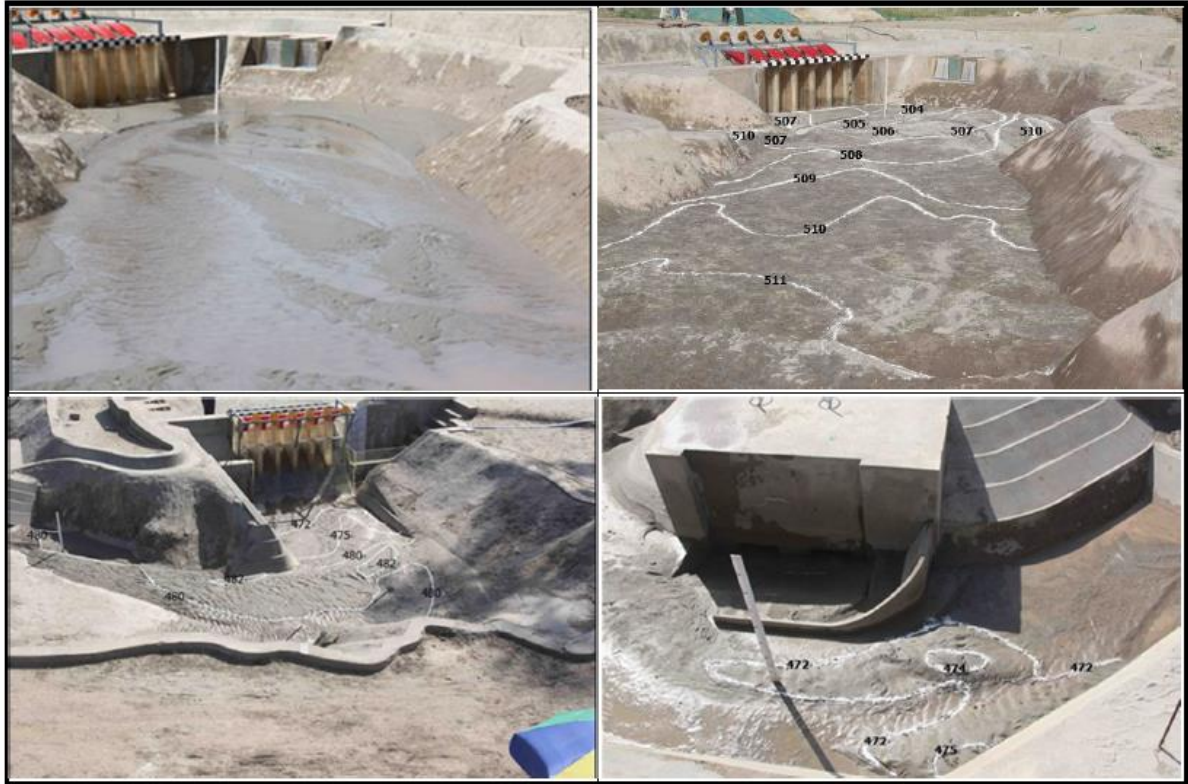
Figure 4.9: Case 3 – Flushing-affected area and sedimentation
