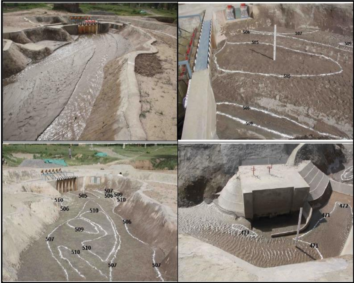
Figure 4.8: Case 2 – Flushing-affected area and sedimentation
