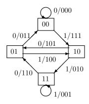
2) The diagram used to find the transfer function of the code is depicted in the next figure
