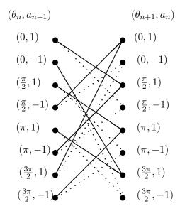
The following is a sketch of the state diagram of the partial response CPM signal.
