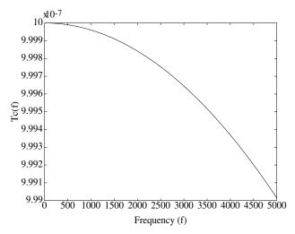
2) The following figure is a plot of the amplitude characteristics of the RC filter, |C(f)|. The values of the vertical axis indicate that |C(f)| can be considered constant for frequencies up to 2000 Hz. Since the same is true for the envelope delay, we conclude that a lowpass signal of bandwidth  $\Delta f = 1$  KHz will not be distorted if it passes the RC filter.
