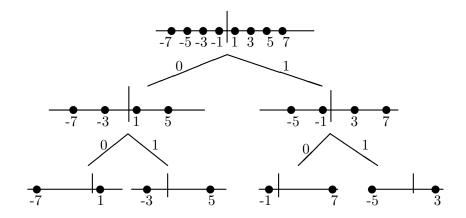
2) The next figure shows one frame of the trellis used to decode the received sequence. Each branch consists of two transitions which correspond to elements in the same coset in the final partition level.
