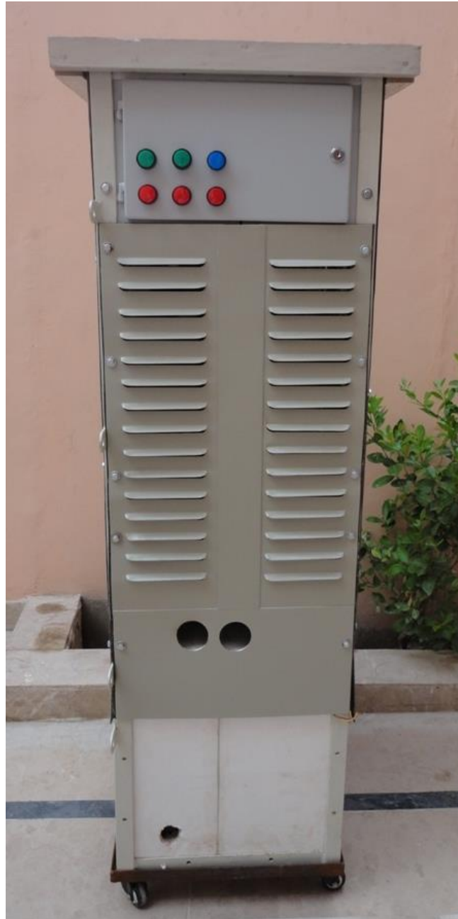
Fig 3.11: A view of dual compressor air-conditioner
