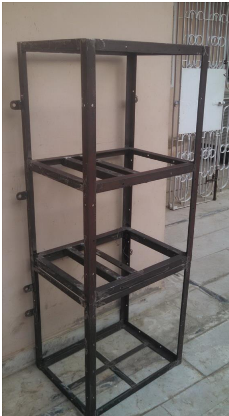
Fig 3.7: Angle iron frame raw form
