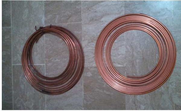
Fig 3.4: Copper Tube used for making Refrigerant (Chilled) Helical Copper coil
