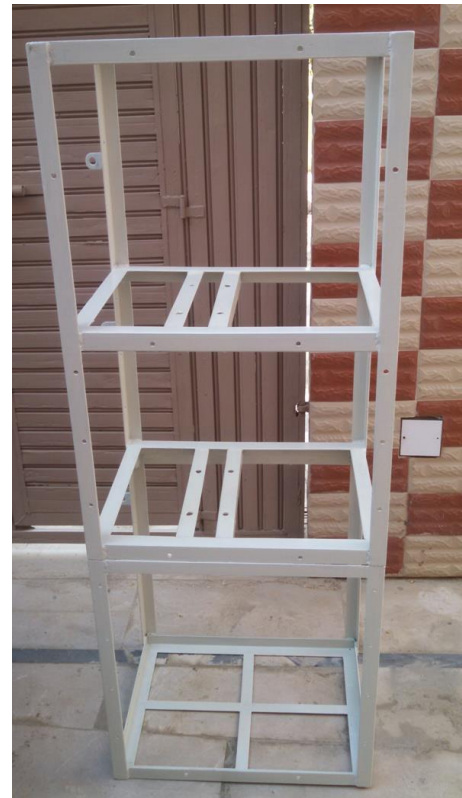
Fig 3.8: Angle iron frame after finishing
