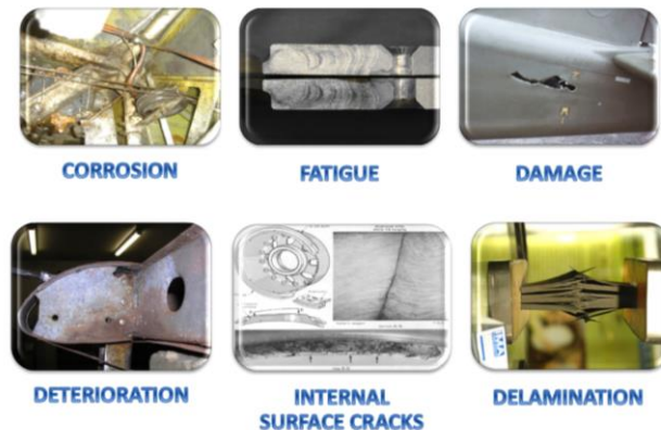
Fig 1-1 Common Aerospace defects
