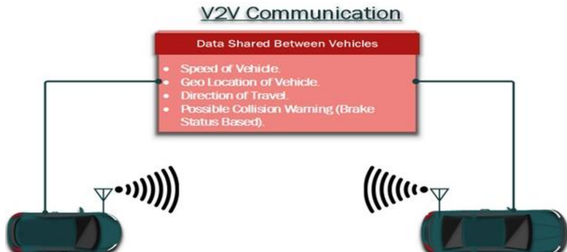
Figure 2.3: Shared data in V2V communication
