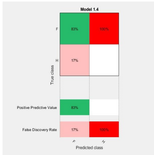
Figure 7.21: Internal Fault - Positive Predictive Values & False Discovery Rates of SVM at Wavelet Band-6
