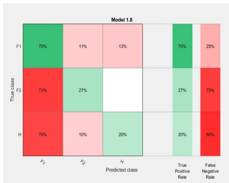
Figure 7.26: Multiple Fault - True Positive & False Negative Rates of SVM at Wavelet Band-6
