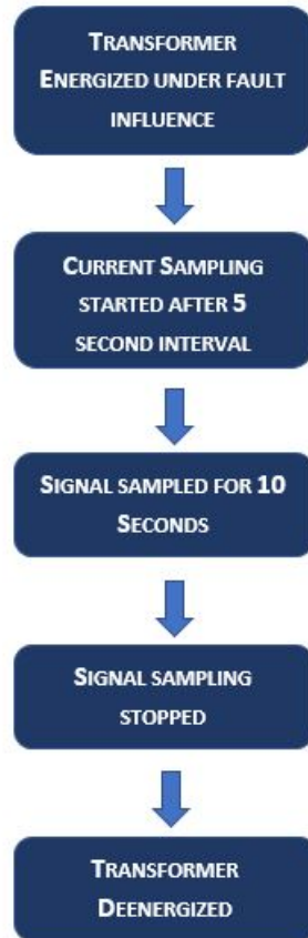
Figure 6.2: Algorithm Flow - Fault Sampling
