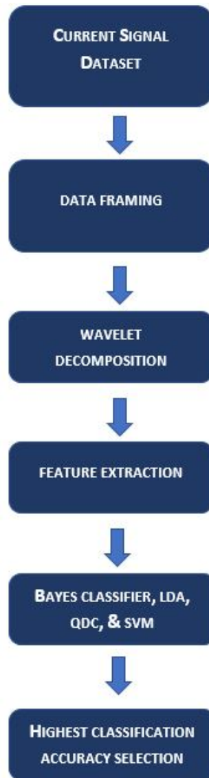
Figure 6.3: Algorithm Flow - Classification
