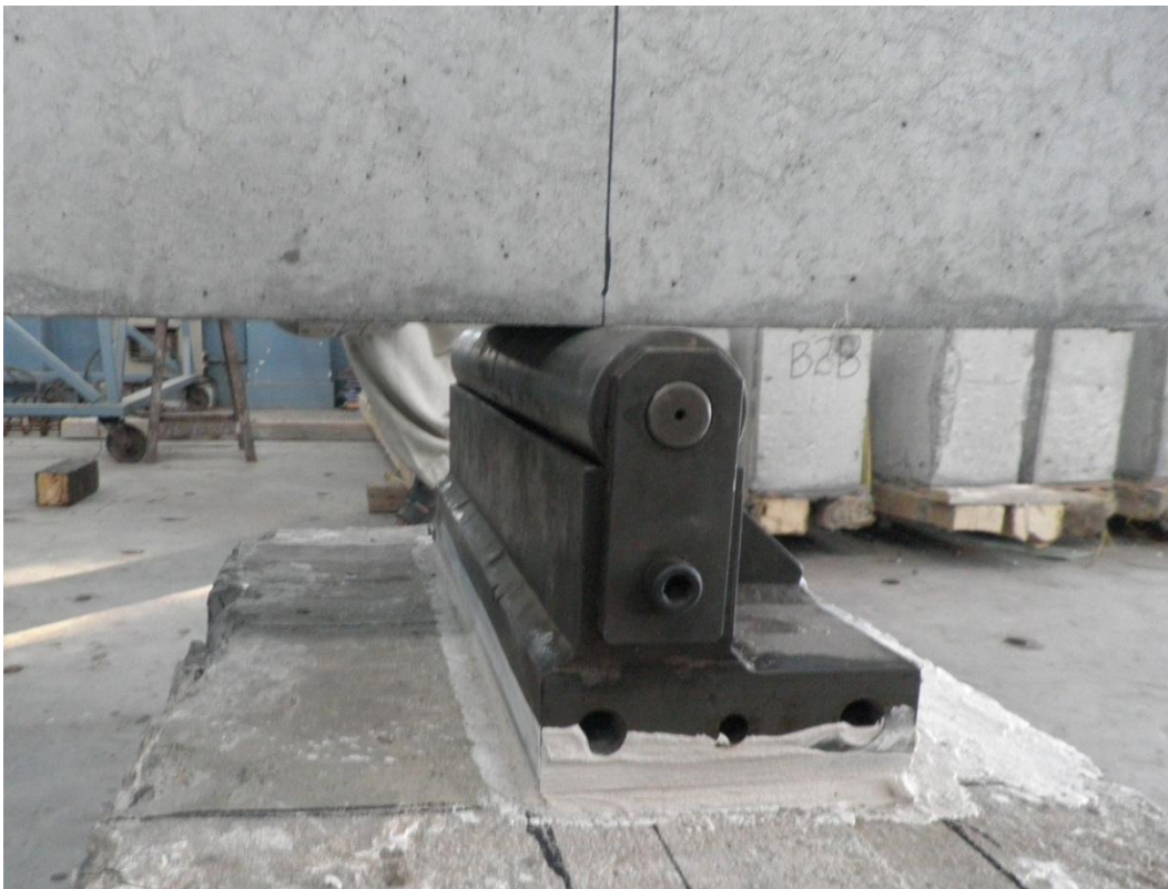
Fig 3.5 Test Setup (Supports)
