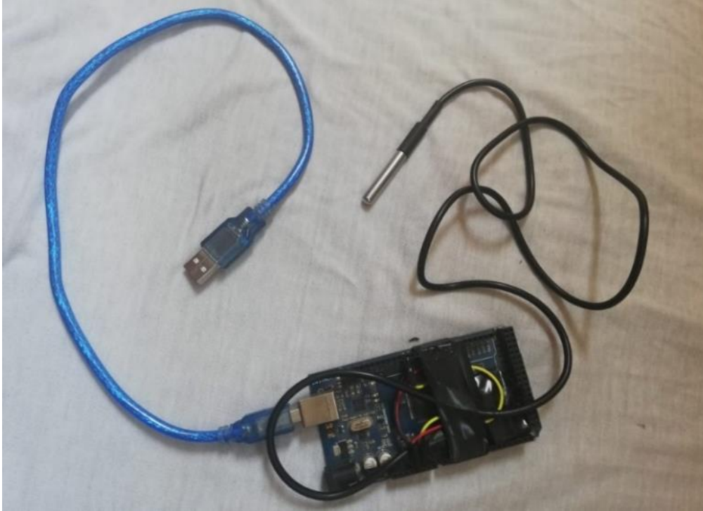
Figure 8: Arduino Mega 2560 with DS18B20 Temperature sensor Sensor, which connected and programmed with Arduino, were carefully placed into the coolant in order to record the difference in temperature. The datasheet of this DS18B20 are given below [52]:
