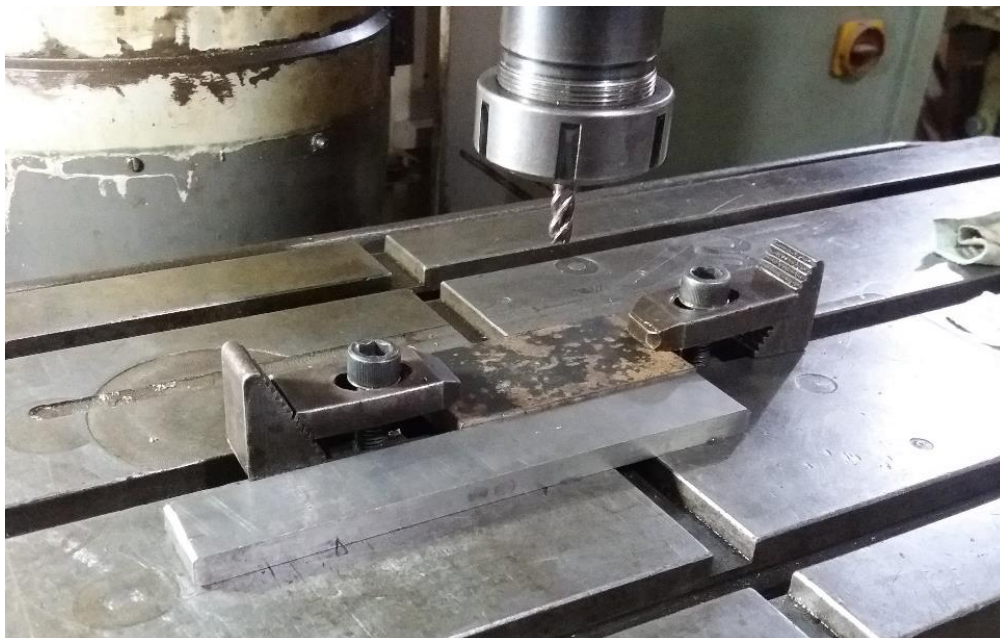
Figure 10: Workpiece clamp for wet machining
