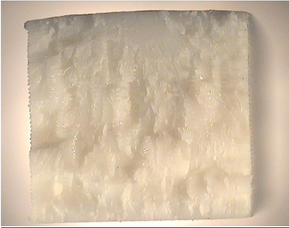
Figure 4.16: Vertical Un-notched specimen with 100% infill density (4UV)
