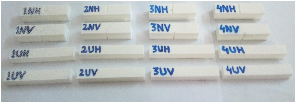
Figure 3.8: Samples Manufactured for Impact Testing (1 Set)
