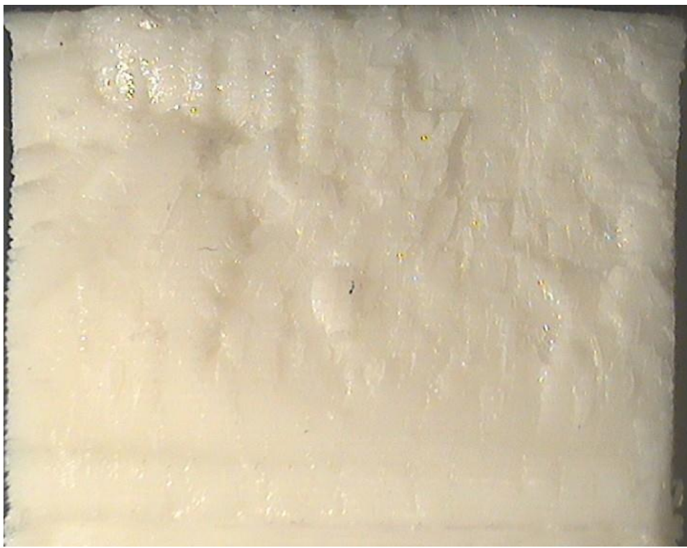
Figure 4.13: Horizontal Notched specimen with 100% infill density (4NH)
