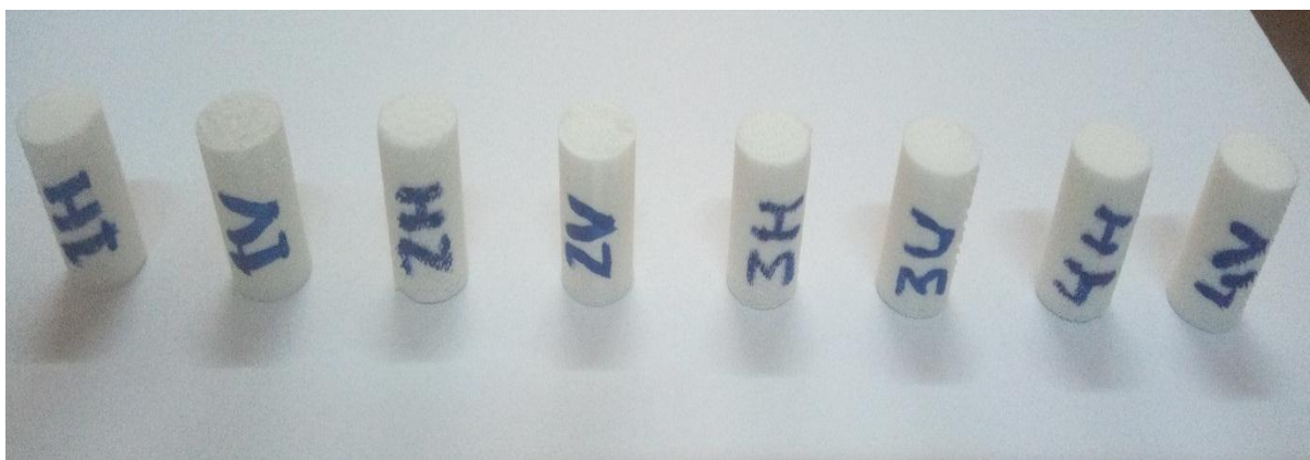
Figure 3.9: Samples Manufactured for Compressive Testing (1 Set)
