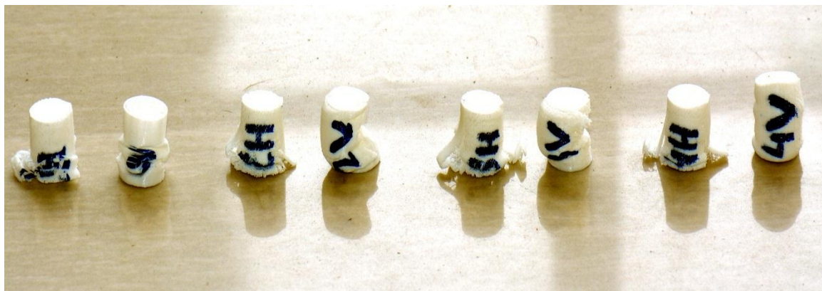
Figure 3.13: Samples after compressive testing
