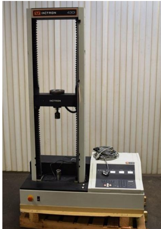
Figure 3.12: Compressive Testing Machine (Instron Model 4301)
