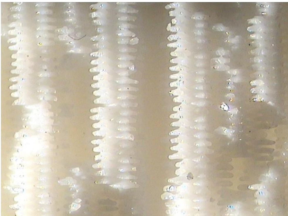
Figure 4.11: Horizontal Un-notched specimen with 75% infill density (3UH)
