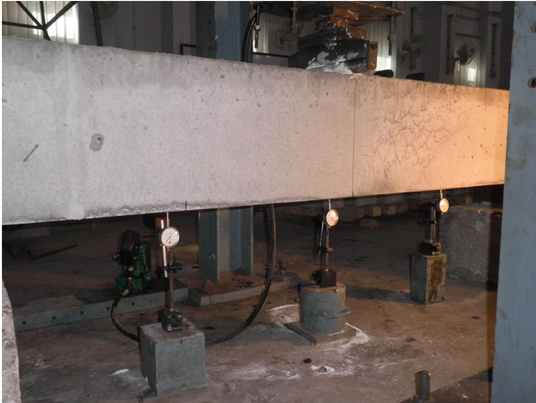
Fig 3.7 Test Setup (Deflection Gauges Placed at Third Point)
