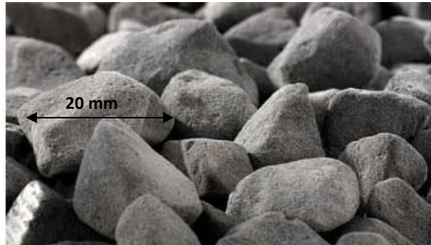
Fig 3.2: Glass Foam Gravels as purchased from GLAPOR [80]
