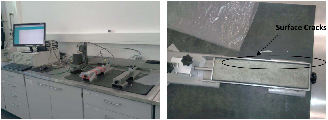
Fig 3.9: Modified German Shrinkage Channel “Schwindrinne” on the left, some shrinkage cracks visible on the specimen on the right
