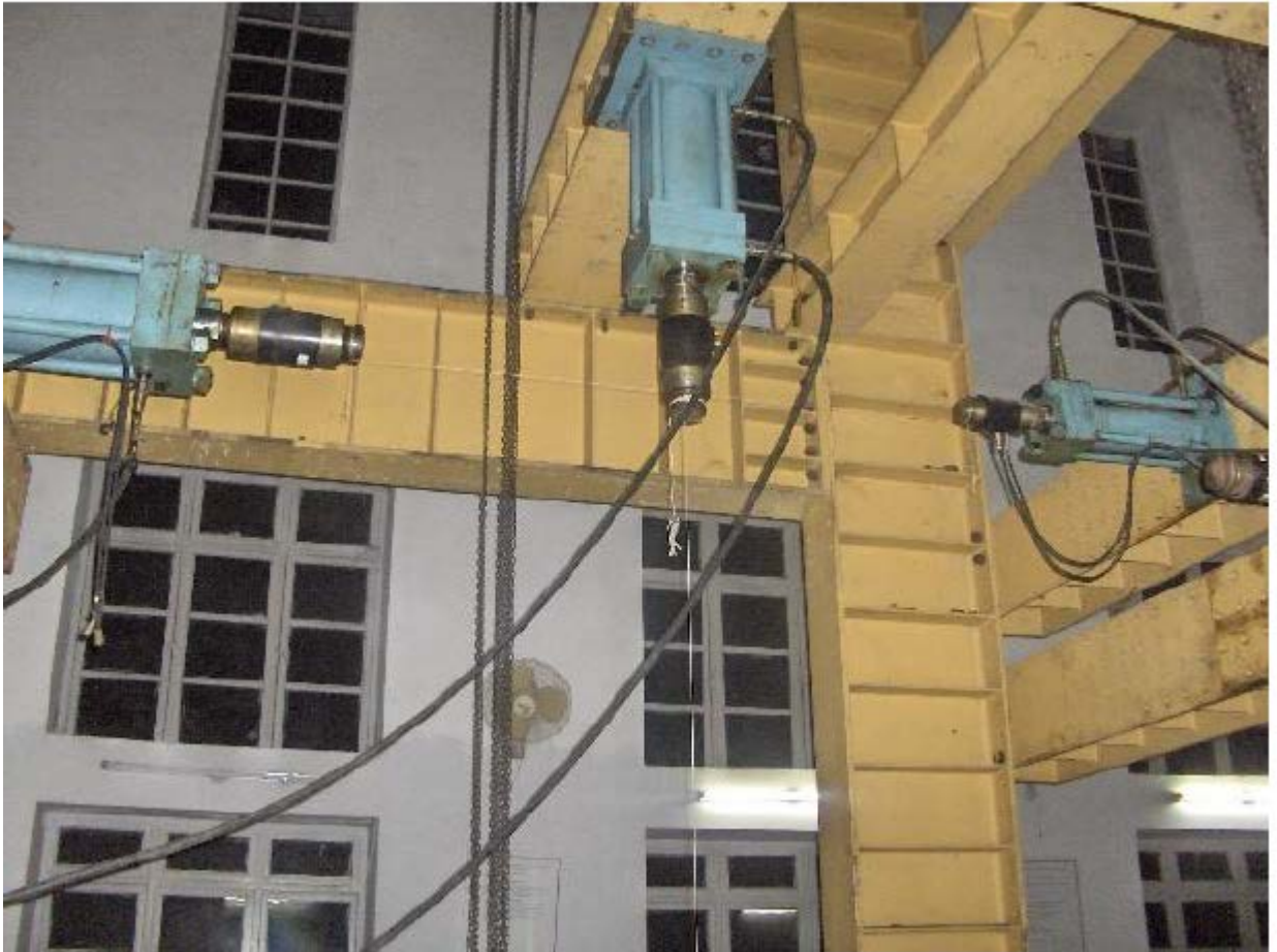
Figure 3.5: Hydraulic actuators in its original form with fix base suitable for monotonic testing for pushing only
